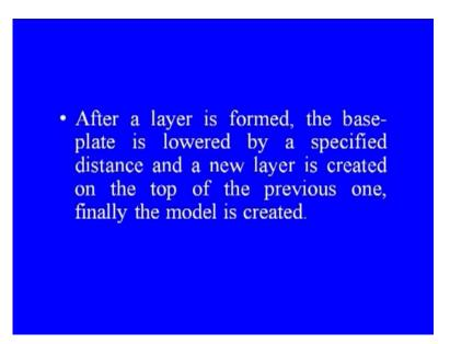
After a layer is formed the base plate is lowered by a specified distance and new layer is created on the top of the previous one. Finally, the model is created then the rapid manufacturing process R M process. So, this can be considered as an extension of rapid prototyping technology, it involves a automatic production of parts by instructions directly fed by the cad data which is modeled earlier.
