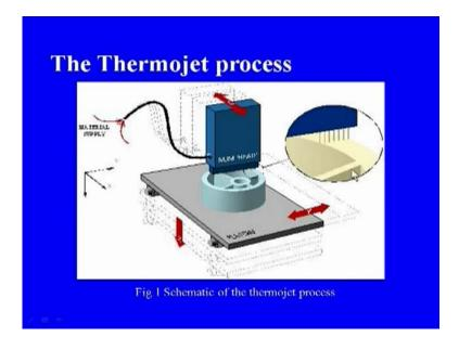
Here this is the platform and this is the object being manufacture and as I have indicated at the very beginning, this is the layer by layer manufacturing process in most of the cases. So therefore, the material is getting deposited on this product and this platform will be lower in a stage, so that next layer can be deposited on top this and top of this. So, if was this layer is being produced then this is lower by a thickness equivalent to the next layer to be produced.
