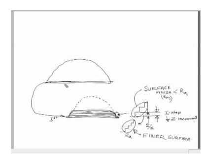
Say for example, this is the parts to be produced now this part will be produced in the rapid prototyping concept, like this first one layer will be produced. On top of this so this layer first layer is being produced, this is a first on top of this the next layer can be produced. So, next layer will be produced, say like this. Next layer will be produced, like this next will be produced on top of this like this.
