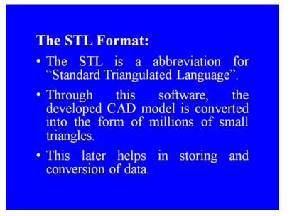
Now, let us see, what is a STL format? The STL is a abbreviation for standard triangulated language. Through this software the developed CAD, CAD model is converted into the form of millions of small triangles. This later helps in storing and conversion of data.
