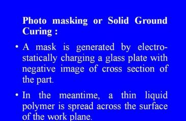
A mask is generated in this process by electro statically charging a glass plate with negative image of cross section of the part. In the meantime, a thin liquid polymer is spread across the surface of the work plane.
