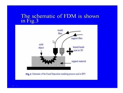
This is being showed in the screen. This is the support material and this is the solid object being produced. So, this is where the model fiber is coming and this is the support fiber that means it provides mechanical support to the model, so that distortion is prevented or minimized to be fair enough. And for scanning there will be a t d, 3 D control mechanisms will be there which will guide these heads in all three directions.
