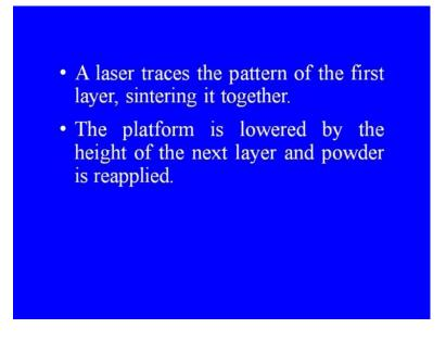
A laser traces the pattern of the first layer, sintering it together. The platform is lowered by the height of the next layer and the powder is reapplied as I have already indicated.
