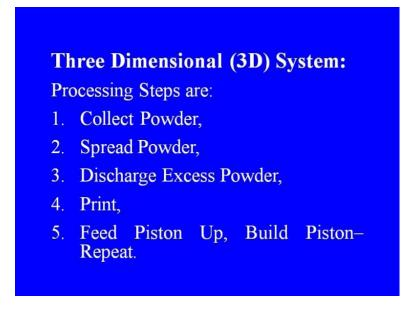
In this 3D process of rapid prototyping system the first step is to collect the powder, spread the powder in a desired shape, then discharge excess powder, then print and then feed piston up, build the piston and we have to repeat this step.
