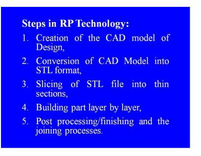
The first step being a CAD model is to be produced, for the design of the product to be produced a cad model is necessary. Then followed by this in the second step this CAD model is converted into STL format that is again the digital phase only. Then this model is sliced into thin sections say for example, if the product height is of 100 millimeter. This is to be sliced; this height is to be sliced into suitable thicknesses, which can be realized in one go of the machine.
