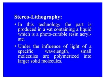
In this technology, the part is produced in a vat containing a liquid, which is a photo curable resin acrylate. Under the influence of light of a specific wavelength, small molecules in this liquid are polymerized into larger solid molecules. This is the basic principle involved in this process. Therefore, the selection of that particular wavelength of light is critical in this process.
