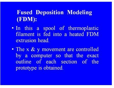
In this a spool of thermoplastic filament is fed into a heated FDM extrusion head. The x and y movement are controlled by a computer, so that the exact outline of each section of the prototype is obtained.
