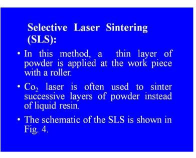
In this method, a thin layer of powders is applied at the work piece with a roller. Carbon di oxide laser is often used to sinter the successive layers of powder instead of liquid resin. The schematic is shown in this figure.
