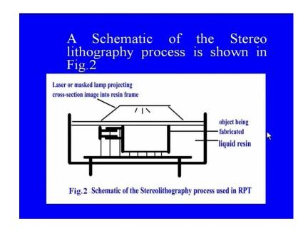
So, this is the schematic on the screen of the stereo lithography process. This is the light emitting device and this is the object being fabricated. This is how the light will fall on the area of interest and this is the liquid, liquid resin which will get solidified or form large molecules under the action of this light, particular frequency of light falling on to it, remaining portions will be masked.
