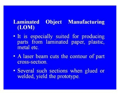
Next, let us discuss another very popular technique that is laminated object manufacturing or LOM technique. It is especially suited for producing parts from laminated paper, plastic, metals etcetera. A laser beam cuts the contour of part cross section. Several such sections when glued or welded, yield the prototype.
