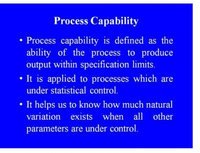
Process capability is defined as the ability of the process to produce output within specification limits, it is applied to processes which are under statistical control. It helps
