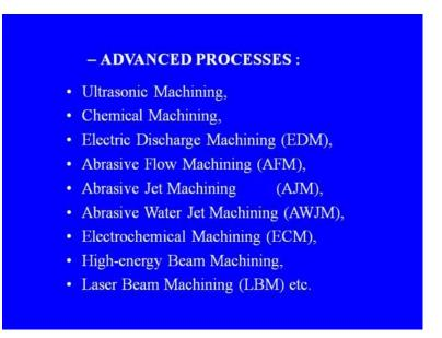
Advanced processes; ultrasonic machining, chemical machining, electro discharge machining, abrasive flow machining, abrasive jet machining, abrasive water jet machining, electrochemical machining, high energy beam machining, laser beam machining etcetera. These processes are also termed as unconventional or nontraditional machining processes. Next major classification is joining.
