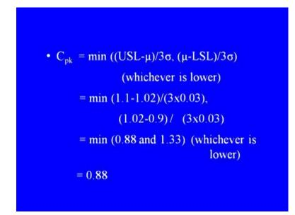
On the other hand C pk for the same situation at the same values given can be calculated as minimum of upper specification limit minus mean by 3 sigma and mean minus lower specification limit by 3 sigma, whichever is lower. And this comes out to be 0.88 with the calculations using those values. Thus the lower one being 0.88 is considered to be the C pk.
