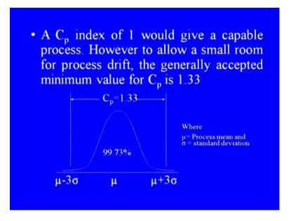
A C p index of 1 would give a capable process. However, to allow a small room for process drift, the generally accepted minimum value for C p is 1.33. This can also be explained with the help of this figure, in which a normal curve, bell curve is shown. And
