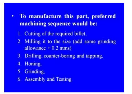
To manufacture this part preferred machining sequence would be, cutting of the required billet, milling it to the size adding some grinding allowance say for example, plus 0.2
