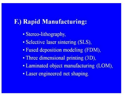
Next category is rapid manufacturing which include; Stereo lithography, selective laser sintering, fused deposition modeling, three dimensional printing, laminated object manufacturing, laser engineered net shaping etcetera. Selection of appropriate process one or more appropriate manufacturing processes amongst the discussed processes are chosen while considering the following factors.
