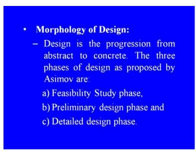
Design is the progression from abstract to concrete, the three phases of design as proposed by Asimov are; Feasibility study phase, then followed by preliminary design phase and finally, the detailed design phase. What are the idea and concepts? The idea initiates from requirements of customers or in some case by the imagination of the designer, to benefit the individual by some means. Developing the idea further requires transforming idea into a concept and further into a product.
