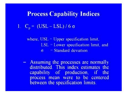
There are number of process capability indices number one, C p. It is defined as the ratio of differences between the upper specification limit and lower specification limit, to the 6 sigma, where sigma stands for standard deviation. Assuming the processes are normally distributed, this index estimates the capability of production. If the process mean were to be centered between the specification limits.
