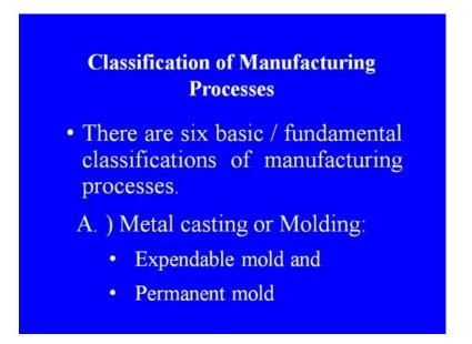
There are six basic fundamental classifications of manufacturing processes. The first metal casting or molding, there are two different approaches in this. Number one expendable mold and number two permanent mold. Next class is metal forming and shearing.
