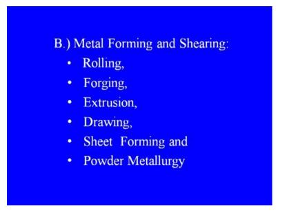
This includes a number of techniques called rolling, forging, extrusion, drawing, sheet forming and powder metallurgy. Next category is material removal, which are also called machining processes. In this there are two broad categories termed as conventional and non conventional.
