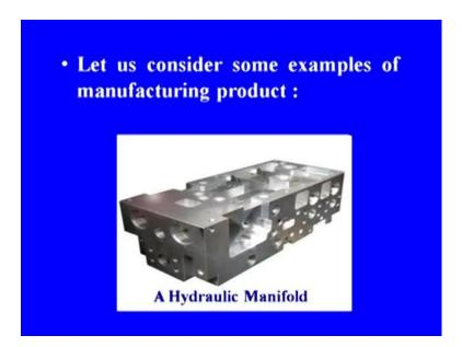
A hydraulic manifold is a classic example of manufacturing product, it is a machined component generally made of mild steal on which valves fittings and houses are seated. It reduces piping to a great extent and is considered as the heart of the hydraulic system. It resembles and integrated circuit of an electronic system machine requirements.
