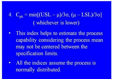
The fourth index is C pk, which is defined as the minimum of upper specification limit minus mu divided by 3 sigma and mu minus lower specification limit divided by 3 sigma, whichever is lower is accepted. This index helps to estimate the process capability, considering the process mean may not be centered between the specification limits. All the indices assume the process is normally distributed.
