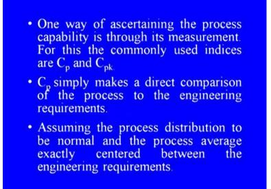
One way of ascertaining the process capability is through its measurement for this the commonly used indices are C p and C p k. C p simply makes a direct comparison of the process to the engineering requirements. Assuming the process distribution to be normal and the process average exactly centered between the engineering requirements.
