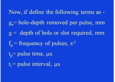
Now, if we define the following terms like g e is the hole depth removed per pulse in millimeter, then g is the depth of the hole or slot required in millimeter, f p is the frequency of pulses per second then t p and t i are the pulse time and pulse intervals in micro seconds. Then the number of pulses required that is n e to remove a hole of depth g, can be described by n e equal to g by g e.
