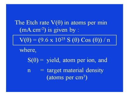
As can be seen in the screen 9.6 into 10 to the power 25 S theta into cos theta divided by n, where S theta is nothing but the yield in terms of atoms per ion, and small n is the target material density, which is atoms per centimeter cube. Then let us see about the accuracy in the surface effects of this ion beam machining.
