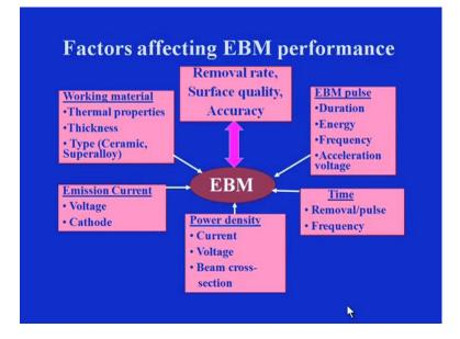
Now, let us see the factors that affect the electron beam machining performance. This factors are generally grouped into these sub headings as shown in the screen, these are work material based parameters in which thermal properties of the material, thickness of the work material and then type of the work material, whether the work material is of ceramic or super alloy etcetera. That influences the material removal rate because the thermal property.
