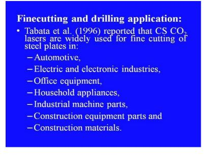
Tabata and his team mates in the year 1996 reported that carbon dioxide lasers are widely used for the cutting of steel plates in, automotive, electric and electronic industries, office equipment, household appliances, industrial machine parts, construction equipment parts and construction materials. The thickness of such cut steel plates range from 0.5 to even up to 16 mm. which is quite thick and the cutting speed carries 6 to 1 meter per minute in different cases.
