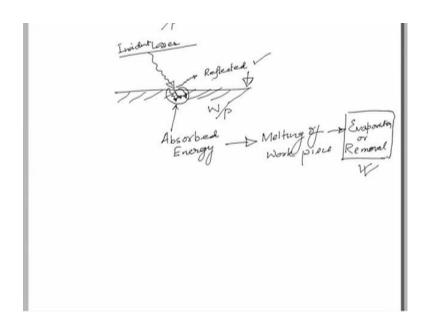
Hence this absorption of the energy by this work-piece material is very, very important rather than getting reflected. So, this would be as less as possible in case of any work-piece that is to be worked with laser energy. The four physical parameters preferred to be lower in magnitude for increasing the process efficiency, as the energy required to melt and vaporize the material is lesser in 1 b m, this we have already discussed.
