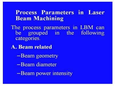
A beam related parameters, this include beam geometry, beam diameter, beam power intensity. This beam diameter and beam power intensity, they play very vital role in the sense that beam diameter will define, how fine we will be able to cut on the work-piece. And beam power intensity will dictate, how intensely we can apply the laser power on the work-piece, and how deep we can go with that power intensity, and how fast we can cut.
