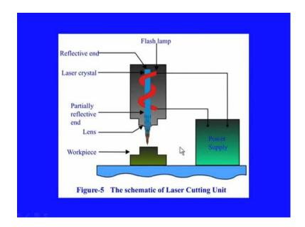
This is another schematic of how the laser is being produced. So, this is the lasent and then this is here that spiral red element is responsible for the additional energy which is in the form of a flash lamp. And this will supply energy to this lasing material and in one end of this mirror system which is partially reflective, therefore some amount of beam will come out as the laser beam and they will be focused with certain lens system on the work piece.
