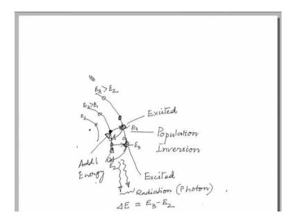
Say for example and in a configuration where electrons are there in different cells. Now, if this electron, this electrons are supplied with some additional energy, additional energy. So, this energy is pumped to this then these electrons from low energies so here this energy level E 1 and this is E 2 which is greater than E 1 and this energy level at this cell is E 3 which is greater than again E 2 that means these electrons at this shell will have the highest energy level.
