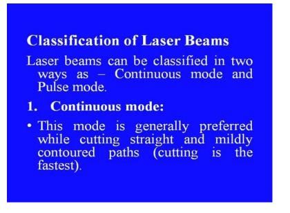
Now, let us look into a classification of laser beams. Laser beams can be classified in two ways continuous mod and pulse mode. Number one continuous mode; this mode is generally preferred while cutting straight and mildly contoured paths, cutting is the fastest. (Refer Slide Time: 22:31)
