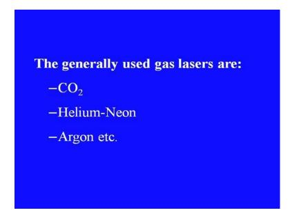
The generally used gas lasers are carbon dioxide laser, helium neon laser and argon laser etcetera. Let us see characteristics of carbon dioxide lasers, these lasers can be operated continuously and on a pulsed basis. Thus, they have wider application in case of continuous mode or in case of pulsed mode.
