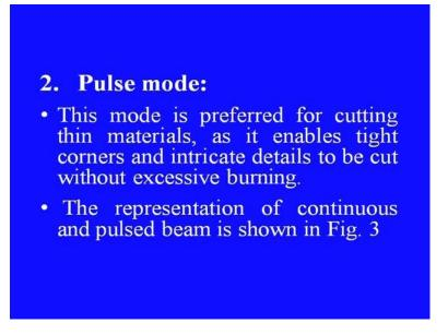
And number two, pulse mode. This pulse mode is preferred for cutting thin materials as it enables tight corners and intricate details to be cut without excessive burning. The representation of continuous and pulse beam is shown in figure three.
