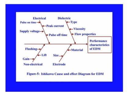
These process parameters are grouped into four main categories electrical parameters, which are pulse on time, supply voltage, peak current and pulse off time. And dielectric based parameters like type of dielectric, viscosity and then flow properties. Then other
