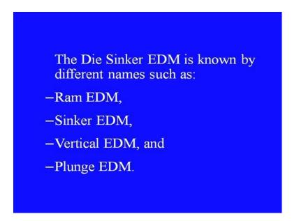
The die sinker EDM is also known by different names such as ram EDM, sinker EDM, vertical EDM and plunge EDM. The insulating liquid used in die sinker EDM completely submerges the electrode and the work piece. Some special oils, special
