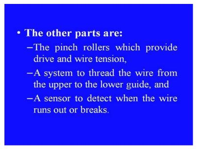
Other parts in this setup are; the pinch rollers, which provide drive and wire tension, a system to thread the wire from the upper to the lower guide and a sensor to detect, when the wire runs out or breaks. Now, let us look into the process parameters in WEDM process, these parameters are shown in this familiar figure.
