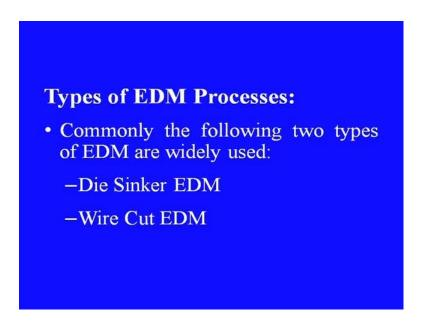
Let us move ahead, in the very beginning let us see the different types of EDM. Commonly there are two types of EDM processes, one is die sinker EDM and the other one is known as wire cut EDM also in short known as WEDM. Let us look into the die sinker EDM. (Refer Slide Time: 01:55)
