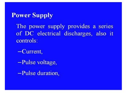
As I have already told the pulse supply the pulse power supply is very important in the case of EDM.
