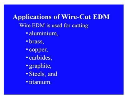
It is used for cutting metals like aluminum, brass, copper, carbides, graphite, steels and titanium. The wire cut materials varies with the application requirements.
