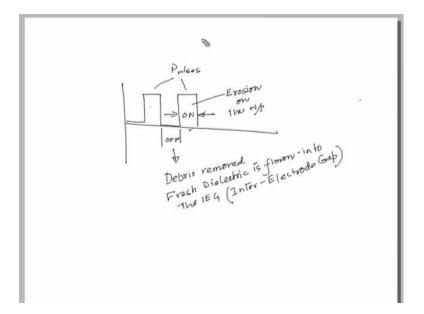
So, this is pulses are like this, like this. So, these pulses, these are known as pulses and this is the off time and this is the on time, of this pulse. During this time, the erosion will take place, erosion on the work piece as well as to some extent on the tool will take place. During this off time, the debris will be removed, debris removed and fresh dielectric is flown in into the IEG, that is known as inter electrode gap. By design we
