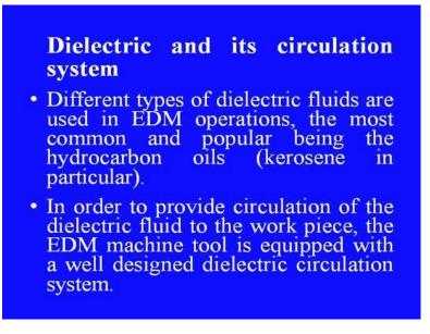
The dielectric and its circulation system also an important subsystem of this entire machining setup, different types of dielectric fluids are used in EDM operations. The most common and popular being the hydrocarbon oils, that is kerosene. In order to provide circulation of the dielectric fluid to the work piece, the EDM machine tool is equipped with a well designed dielectric circulation system. The dielectric circulation system consists of the following two parts, two major parts.
