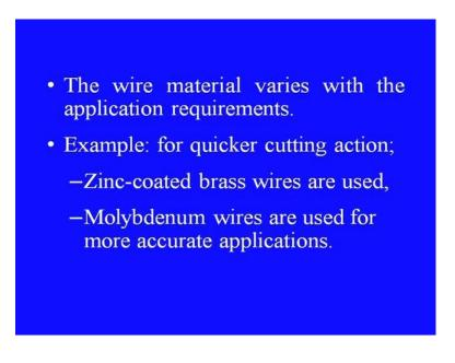
For example, for quicker cutting action zinc coated brass wires are used. Molybdenum wires are used for more accurate applications, the process is used in the following areas aerospace, medical, electronics and semiconductor applications.
