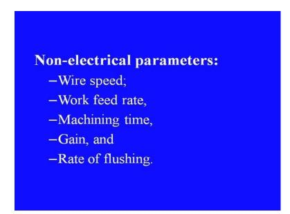
Non electrical parameters include, wire speed, work feed rate, machining time, gain and rate of flushing as well. Whereas, electrode based parameters include, material and size of the wire. The dielectric system based parameters include, type of the dielectric, viscosity of the dielectric and other flow characteristics.
