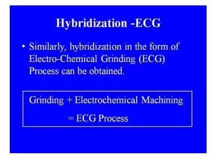
Hybridization in the form of electrochemical grinding ECG process can be obtained. In which conventional grinding will be combined with electrochemical machining, to obtain the electrochemical grinding process. The process is used for machining metallic components, combining these two processes improved productivity and tool life to a great extent.
