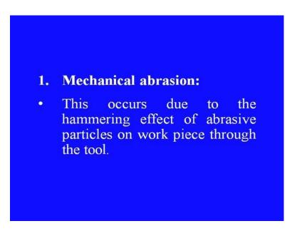
Number one is mechanical abrasion. This occurs due to the hammering effect of the abrasive particles on work piece through the tool.
