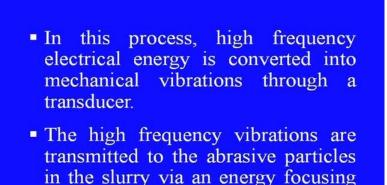
device or horn/tool assembly.
