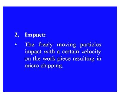
Number two is the impact. The freely moving particles impact with a certain velocity on the work piece, which results in micro chipping on the work piece surface.
