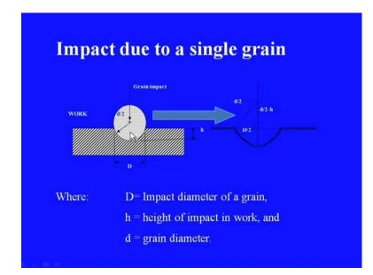
It is being hammered on this work piece. Suppose, this is being inserted or it is indenting the work piece by a distance something like h, the diameter of this particle is say d and the diameter here at at the impact point the maximum diameter is capital D. Then the geometry can be represented something like this, so this is the D by two distance and this is small d by 2 minus the height of the indentation, this is the height of the indentation. (Refer Slide Time: 22:51)
