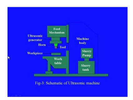
So, this is the overall structure of the of the setup and this is the work table on which the work work piece is been clamped and this is working head also as the tool. This is where the ultrasonic generating facilities will be located and ultrasonic frequencies will be transmitted through the horn assembly or the clamping device to this tool. So, ultimately we will be observing the mechanical oscillations or displacements of this tool head at this point.
