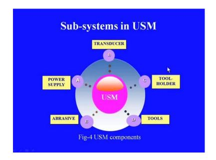
So, these are the main subsystems effecting this ultrasonic machining system. The transducer, which produces, which is responsible for producing the ultrasonic frequency. The tool holder, which is responsible for giving a reseed clamping of the tool and transmitting the the frequency from the transducer to the tool head. Then the tools, the tool itself, which will be responsible for producing the accurate feature on the work piece. The tool will be as per the requirement of the job.
