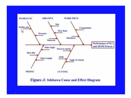
This parameters are hydraulic based parameters like orifice size and orifice and the pressure and fluid pressure. Then abrasive jet parameters are like size of the abrasives, then flow rate, then the material abrasive material itself, which can be silicon carbide or aluminium oxide etcetera and higher the abrasive size, then there will be rate of cutting will be better. But of course, we have to see the life of the nozzle here, which will go down, then the work piece, work piece material.
