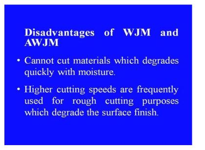
It cannot cut materials, which degrades quickly with moisture because water is essentially lead a component, which is responsible for cutting. Higher cutting speeds are frequently used for rough cutting purposes, which degrade the surface finish.
