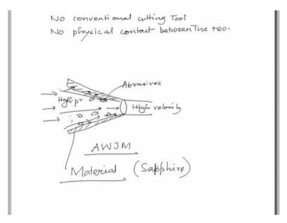
As I told earlier this jet is the very crucial component in this entire set up. Since, the water will be coming through this at very, very high pressure, at this stage it will be of high pressure. At this stage while discharging it will be of very high velocity, therefore
