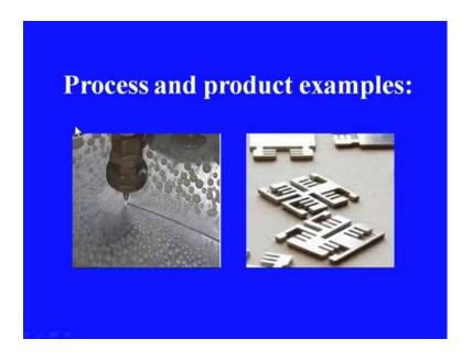
This is typical product that is being produced by or cut by water jet machine. This is the machining head, which cuts like this and here the job is fed rather than the head cutting head. This is the cutting head, through which the pressurized water is coming out and causing the cut or slit. The final product may be something like this or of different
