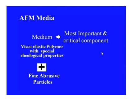
Here is the method how the media is prepared. First of all as I said visco-elastic polymer is taken with special rheological properties that is viscosities, and then added to it is the fine abrasive particles. Of course, their fineness is to be determined or decided as per the requirements, like for getting very high surface finish we have to use fine abrasive particles and so on.
