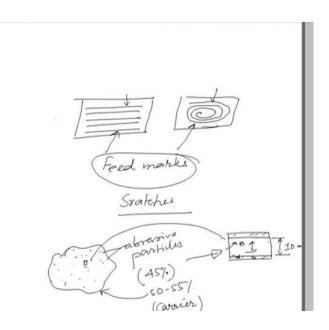
The media if it is something like this which is very soft, highly viscous media and this contains some of the abrasive particles, these are the abrasive particles, these are abrasive particles. Now this abrasive particles at some percentage, say for example, say 45 percent and remaining 55 percent, 50 to 55 percent is say the carrier. This is also called
