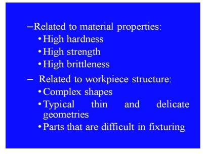
Then related to the work piece structure if the shapes are very complex, then giving these shapes by conventional machining processes is surely time taking. Then typical thin and delicate geometries of the jobs that also takes lot of production time and hence the cost of production gets increased with these conventional processes. Then parts that are difficult in fixturing, this is another important aspect, as we know in case of the machines like lathe, milling, grinding etcetera.
