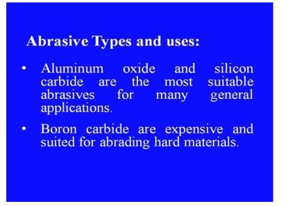
Then what are the different abrasives used in this particular process. As I said already aluminum oxide is by far the mostly used abrasive material along with silicon carbide. Almost all general applications these two types of abrasive materials are used. However boron carbides are used in some machining of some hard materials, but they are very expensive.
