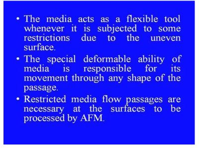
The media acts as a flexible tool whenever it is subjected to some restrictions due to the uneven surface the special deformable ability of this media is responsible for its movement through any shape of the passage this can be seen like this.
