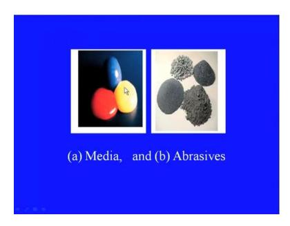
Here are some of the like carrier, and these are some of the abrasives used in this process, they are mixed together uniformly and that forms the working media. The
