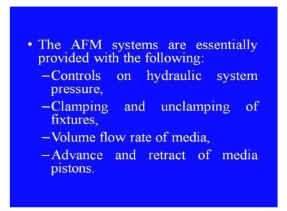
The AFM systems are essentially provided with the following things like controls on hydraulic system pressure, the clamping and unclamping of the fixtures, the volume flow rate of media, the advance and retract of media pistons.
