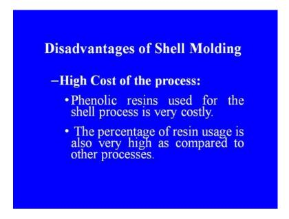
The phenolic resins used in this process is very costly. The percentage of resin usage is also very high as compared to other processes, which adds to the high costs of the process. The process also requires very tight control of the shell thickness; else the competitiveness of the process will be sacrificed. Smaller shell thickness limits the weight of the castings that are produced by this process. Producing bulk air castings can lead to shell breakages as it cannot bear more weights.
