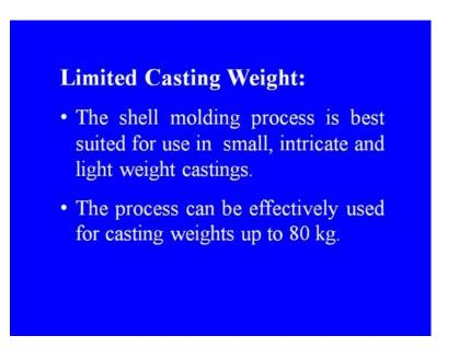
Limited casting weight, the shell molding process is best suited for use in small, intricate and light weight castings. The process can be effectively used for casting weights up to 80 kilograms.
