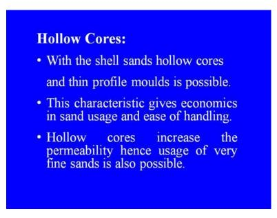
Next is the hollow cores, with the shell sands hollow cores, the thin profile moulds is possible. This characteristic gives economics in sand usage and ease of handling. Hollow cores increase the permeability and hence usage of very fine sands is also possible. Sand to metal ratio, this is a unique process that gives hollow cores and thin wall moulds. The hollow cores help in improving the permeability and act as a basis for the evolved gases
