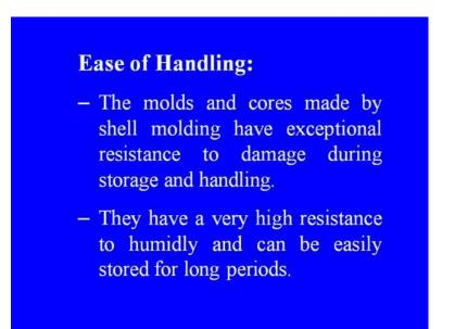
Ease of handling is another big advantage of this process. The molds and cores made by the shell molding have exceptional resistance to damage during storage and handling. They have a very high resistance to humidity and can be easily stored for long periods.
