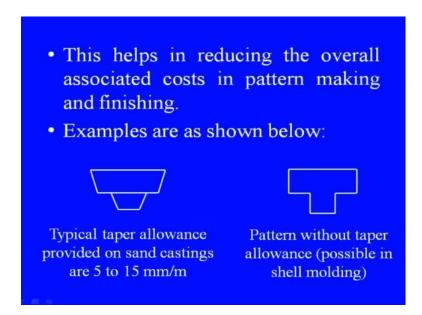
This helps in reducing the overall associated costs in pattern making and finishing. The examples are given here, this is a typical taper allowance, this is a pattern with taper
