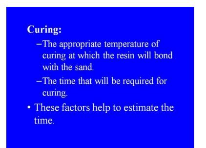
Then the importance of curing, the appropriate temperature of curing at which the shell will bond with the sand, the time that will be required for curing. These factors help to estimate the time. Now, let us look into the functions of additives. Additives may be added to the sand aggregate to further enhance the surface finish of the casting. It also improves the strength of the mold, and develops the resistance to thermal cracking and distortion.
