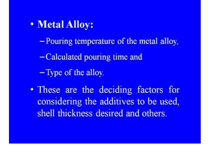
These are pouring temperature of the metal and alloy, then calculated pouring time and type of the alloy. These are the deciding factors for considering the additives to be used, shell thickness desired and others. Then in the category of additives this use of correct additive and its composition is decided considering the following factors.
