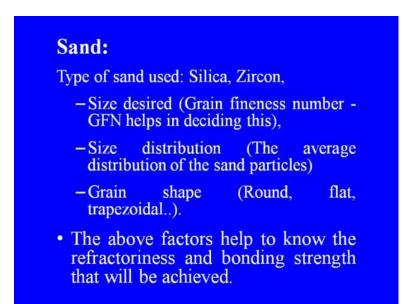
The type of sand used in shell molding are silica and zircon. So, they depend on the size desired then in this size the factor which is considered is GFN that is grain fineness number that helps in deciding the size. Then size distribution, the average distribution of the sand particles then the grain shape where they are round, flat or trapezoidal.
