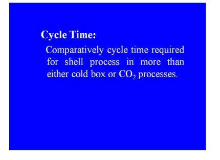
Cycle time, comparatively cycle time required for shell process in, is more than either cold box or carbon dioxide processes.
