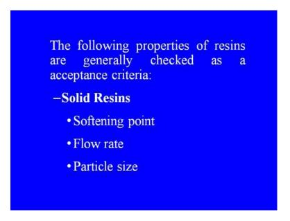
The following properties of resins are generally checked as a acceptance criteria for solid resins, softening points, flow rate and particle size.
