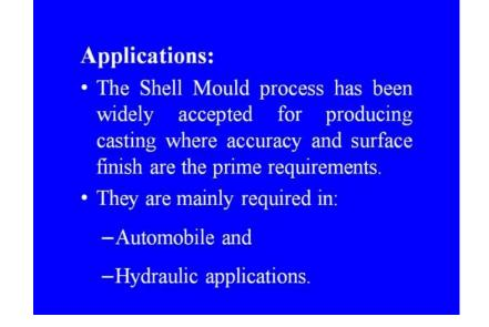
The shell molding process has been widely accepted for producing castings where accuracy and surface finish are the prime requirements. They are mainly required in automobile and hydraulic applications. Small mechanical parts requiring high precision such as gear housings, cylinder heads and connecting rods, these components can be manufactured by the shell molding process.
