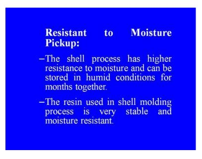
Resistance to moisture pickup this is another big advantage. The shell process has higher resistance to moisture and can be stored in humid conditions for months together. The resin used in shell molding process is very stable and moisture resistant.
