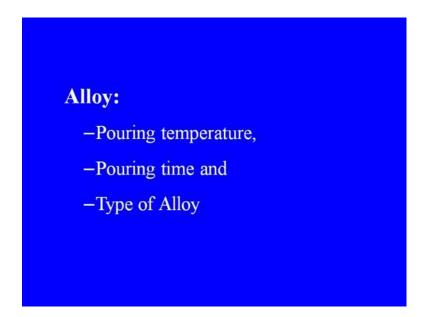
Then alloy, parameters that is pouring temperature pouring time and type of alloy. Then regarding ceramic slurry pH value of the slurry, density of the slurry and viscosity of the slurry are the parameters of major interest.
