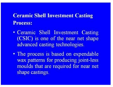
In this process a near net shape product can be produced. This is very widely used technique now a days.
