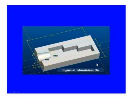
And this is the aluminum die in which this three step mould is created.
