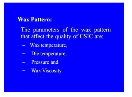
The wax patterns, the parameters of the wax pattern, that affect the quality of ceramic shell investment casting are wax temperature, die temperature, pressures and wax viscosity. Of course, then stucco based parameters, that are the type composition size and size distribution.
