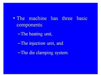
The machine has three basic components. the heating unit to maintain the temperature. the injection unit and the die clamping system. This machine has the following essential components and provisions a jacket provided for heating and melting of the wax that occurs in an aluminum reservoir with provision for slow speed, staring injection of the liquid wax from the brass cylinder under pressure into a closed mould.
