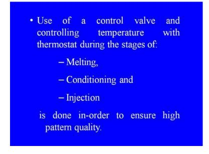
Use of a control valve and controlling temperature with thermostat during the stages of, melting, conditioning and injection is done in order to ensure high pattern quality.
