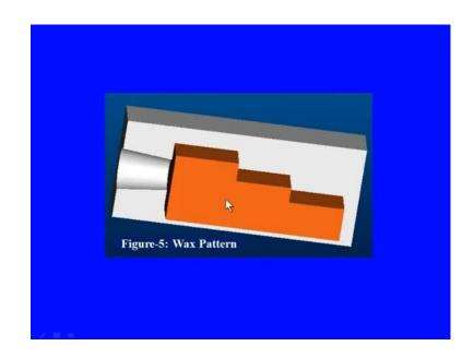
This is the wax pattern. Now, let us see some details about a wax injection machine. A wax injector is a machine, which makes use of an earlier conditioned wax and injects it into a die. In order to produce our wax pattern and injection machine was design and fabricated at IIT Roorkee and is shown in figure six.
