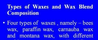
and montana wax, carnauba wax and montana wax, with different melting temperatures (58.2°C to 83.8°C) can be used to make the pattern suitable for use in investment and ceramic shell investment castings.
