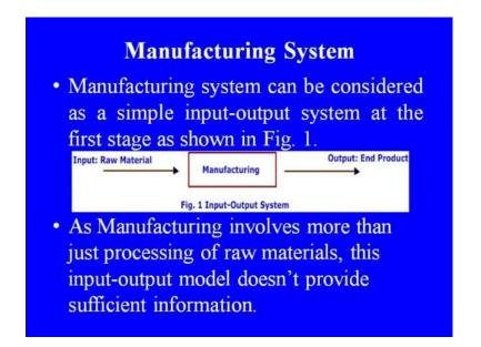
A manufacturing system can be considered as a simple input-output system at the first stage as shown in the figure 1. As manufacturing involves more than just processing of raw materials, this input-output model does not provide sufficient information. Manufacturing as a system involves other inputs like energy, planning, appropriate missionaries and product or customers' requirements apart from raw materials.
