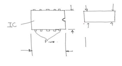
Planarization is can be considered as a common process. In which all I C's are having some shape something like this. So, here that connecting button should be or connecting pin should be there, these are known as pins. So, these are pins and this is the body of the I C, in which number of circuits will be there integrated and this for orientation. Now, in this, this planarization that means the I C should be as for as the dimension is concerned.
