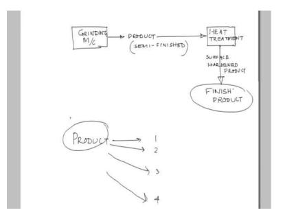
Then this whatever, we are getting the output from the grinding machine, say grinding machine. So, this is the product so this product again we can say so this is a semi finished. Semi finished product only, because it does not meet the criteria of the hardened surface. So, therefore we may need to take this semi finished product to some heat treatment, say heat treatment process in which the surface hardening will be done and that product with surface hardens.
