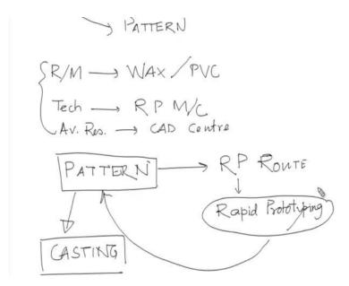
However, in the same situation if the things are say. For example, as raw material I have raw material is say wax or some other say P V C material, then I have the technique available, say technique available is say rapid prototyping technique or the machine I am having is the rapid prototyping machine. Then probably with these requirements and techniques available probably I will go for the same pattern making, pattern and of course, I have say available in available resources.
