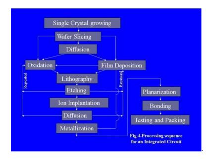
So, the process sequences some generalized process sequences. There may be more number of operations in it or may be some operations can be shortened also or cut down also from these sequences, but this is let us consider, this as a generalized process sequence of manufacturing of an I C. So, first and foremost requirement is we need a single crystal so that is considered as the first thing.
