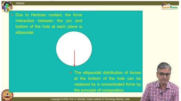
And this force interaction is elliptical distribution. This is done by Hertz. And you model this as by a resultant as a single concentrated force.
