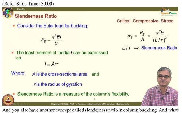
And you also have another concept called slenderness ratio in column buckling. And what you do is, you write the moment of inertia as  $I = Ar^2$ , where *r* is the radius of gyration. So, instead of looking at that as a critical load, I can also get that as critical stress
