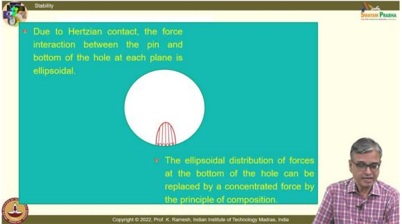
So, when I have a pin, you always have deformation. Even though in rigid body mechanics, we say it is rigid, you have deformation, you have force interaction.
