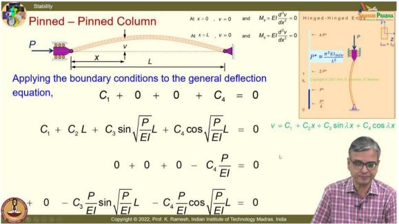
And first, we have looked at the fixed-free, that is the cantilever; then we moved on to pinned-pinned column. And actually pinned-pinned column forms the basis. See, if you look at the critical load, I have also put this as
