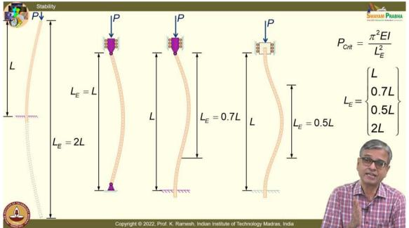
I am now going to discuss the concept of equivalent length, ok. So, I take the pinnedpinned column as the basis. I call this as  $L_E = L$ . I can also visualize, see if I have a longer column, it is dangerous. A shorter column is better. That is the way you have to look at it. Longer the column, its tendency to buckle is more; Its tendency to buckle is more. If I go to fixed-pinned, we have already got the expression. Now, we are going to have a relook
