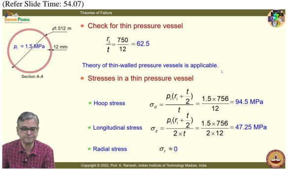
So, first is you have to check for a thin pressure vessel. It is obviously a thin pressure vessel. So, I have this greater than 10; it is about 62.5. And you have a thin pressure vessel is applicable and you know the stresses in a thin pressure vessel. I have a hoop stress. See, usually what they do is, when they do the calculation, they do the calculation for the median line, ok. So, that is what is illustrated in this; pr/t is the basic expression. Instead
