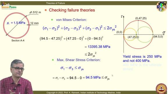
So, the computations are very simple. So, I have the von Mises criteria; you write the von Mises criteria in the basic form, substitute these numbers. And you are in a position to
