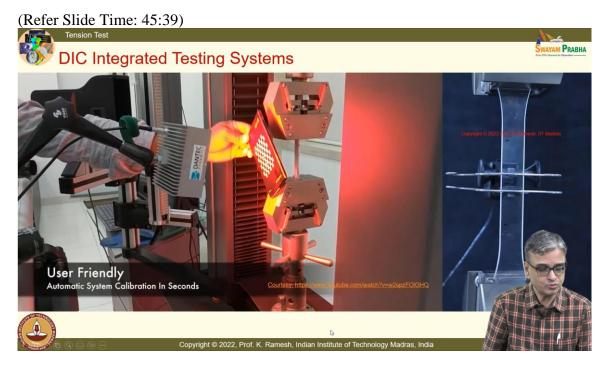
And we have also looked at use of DIC along with tensile testing machine for you to get the data and you can also get true stress and true strain.
