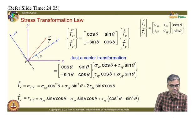
So, you have to do that transformation two times. And we have this stress vector  $\hat{T}$ . And this is simply your rotation matrix. Rest of it, mathematics is simple, you should write the rotation matrix properly. And this is how you have done the tensorial transformation, the second stage is a vector transformation.
