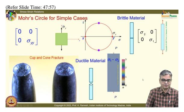
And in a ductile material, if it yields we say that it is yielding and we have also looked at for brittle material, how the failure happens and you are in a position to do that. We have said that this is maximum tensile stress theory and ductile material, it is at  $45^{\circ}$ ; you recognize from Mohr's circle. So, failure happens at  $45^{\circ}$ , that is why you have a cup and cone fracture.
