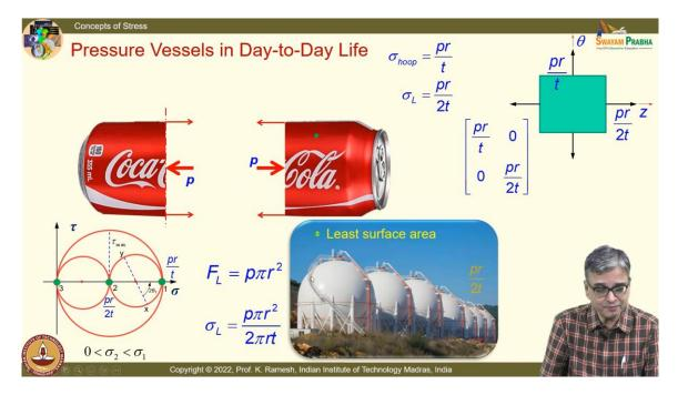
And I said that this is a closed pressure vessel. When I have a closed pressure vessel, I should also worry about what is the force in the other direction. And we have taken a generic cross-section and this is  $F_L = p\pi r^2$ . And I get  $\sigma_L = \frac{pr}{2t}$  and we have got  $\sigma_{hoop} = \frac{pr}{t}$ . And if you take any generic point, it is a true case of a two-dimensional state of stress.
