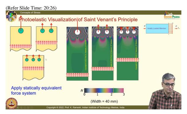
And in the development, we have also discussed a very important principle which is usually talked in the side line in books. So, you have to appreciate what is the Saint Venant's Principle. If I apply an axial load, I can apply it by either a single force or two forces or three forces or even a uniform loading if I am capable of having a grip and pulling it.
