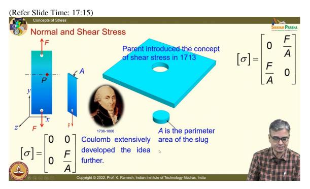
And then we also recognize that stress tensor is tensor of rank 2 and all that. And you know, normal stress was something easier to perceive. So, people were able to understand what is normal stress, which we have looked at from a simple tension specimen. And we have also defined force divided by area as this value.
