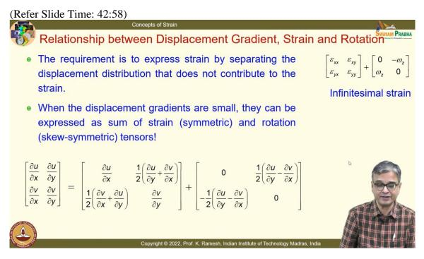
And we have also noted a very interesting relationship between the displacement gradient, strain and rotation. When you have small deformation, this can be put as sum; that is sum of a strain tensor and a rotation tensor. And we have also looked at, this is called infinitesimal strain, because we were looking at small deformation and we have looked at infinitesimal strain.
