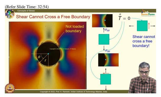
And we have also looked at shear cannot cross a free boundary. We have taken the problem of a plate with a hole and you know this has a very high stress concentration. And we have taken a point on the boundary and we have said that shear cannot cross a free boundary.
