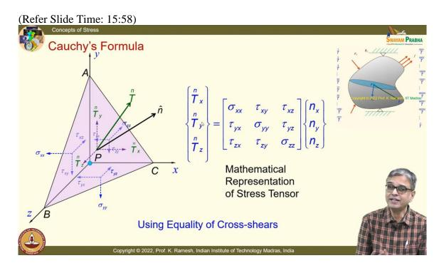
And the Cauchy's formula takes a tetrahedron and then in the limit, shrink it to zero. And we have developed it by invoking the equilibrium conditions. In fact, we have got this as with respect to this column, but we wrote it like this because it is easy for me to write it in a matrix form. And we have utilized the concept of equality of cross-shears to write this. See, in strength of materials, it is very difficult to develop the subject without looking at what is the future development.
