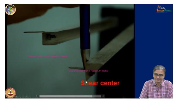
So, I could show the twist better and shear center is very close to this and you find that this is moving straight.
