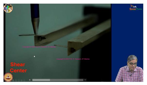
You see a marked difference; don't you see that? So, you appreciate there is something called shear center. I can just make an open section like this to only bend, not twist and *L*-angle.
