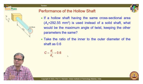
See, the area of cross-section is given right here; we will also calculate. And you have to remember that we have limited the angle of twist as  $0.5^{\circ}$  and we got the diameter as 19.3 mm, fine? And you are also given another simplification. Take the value of  $d_i/d_o$  as 0.6; that is given in the problem statement. Because I can construct multiple hollow shafts even if I want to map the same area of cross-section.
