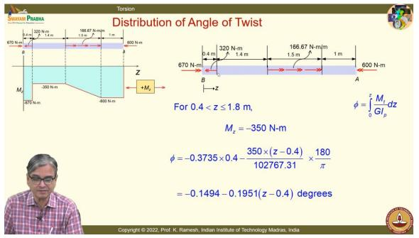
So, here I should have the angle of twist at this end and then bring in what is due to the next one. So, I have z is here and then I start from this, that is 0.4 m to 1.8 m. That is why I have a factor (z - 0.4) coming in here. Then I calculate this, ok? And when I go to the next one, what I will have to do is, I have to do the integration of this, ok? I will just show that and stop for this class.
