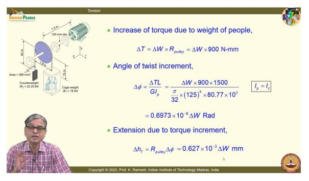
So, increase of torque due to weight of people is  $\Delta W$  multiplied by radius of the pulley and that is also given; you are given diameter as 1.8 m. So, I get this number here. And what is the increment in the angle of twist? So, I have  $\Delta \phi = \frac{\Delta TL}{GI_p}$  and you know what is the  $I_p$  for a circular shaft.
