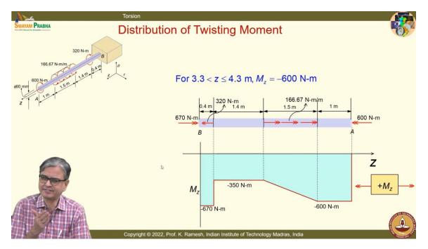
And we have already looked at the twisting moment. I am just going to show this so that we need these numbers for us to calculate. If I want to calculate the angle of twist, I need to know what is the twisting moment at that cross-section.
