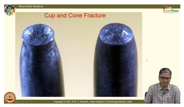
And from our understanding, what is important is how does the failure take place? You have a cup and a cone fracture; this is how it is referred to. So, what happens is, initially you have a crack develops at the center. Because of the brittle failure, it propagates and then finally you have this as shear lips.
