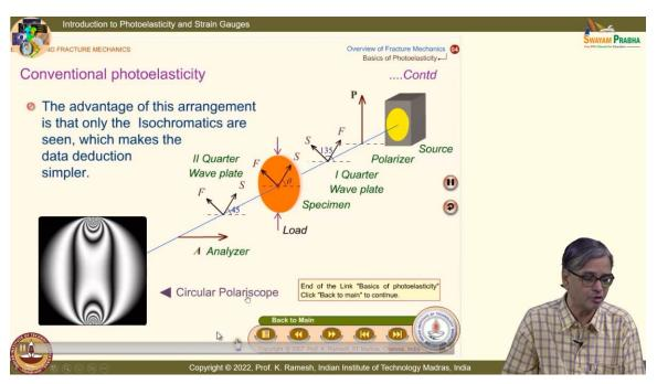
It makes my measurement very very comfortable and easy. In all my earlier slides, I have used only this arrangement to show you fringes. I have not used the monochromatic light source, but I have used the white light source. When I use a monochromatic light source, I will have only this as black and white. And you can also see one more thing. You know if you have this, I have the background as black and I rotate the analyzer, the background becomes white.
