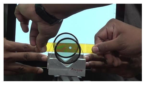
So, at a point of interest, the principal stress directions are behaving like the optic axis, what we have seen in a crystal. And this happens only when it is stressed. When it is not stressed, it will be like a normal material. When I put it, the light will be cut off if the analyzer is perpendicular to that. So, it is beautiful, it is nature's gift to humanity.
