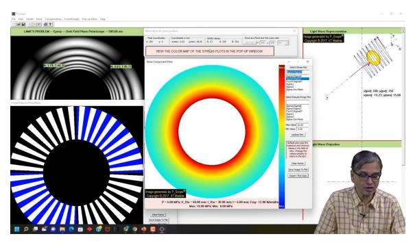
We have determined in your thin cylinder only hoop stress, but here you will have hoop stress as well as radial stress is possible, but we will have this as  $\sigma_{\theta}$ ,  $\sigma_{\theta}$  is plotted like this. Now, the question is you know we have done it for a load of 6 MPa pressure, so what I will do is I will reduce this by 3 MPa that means, I am reducing the load.
