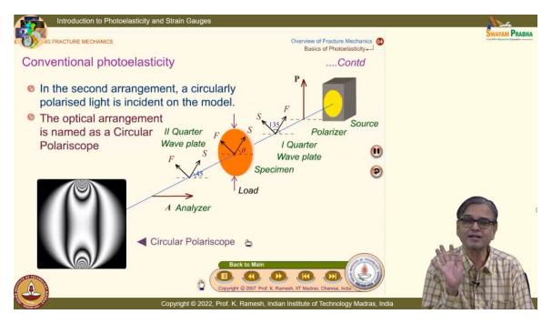
And now, I do not send a plane polarized light, but I put another optical element which will help me to make it circularly polarized. When I send a circularly polarized light, I have a convenient light. I see only one set of fringes.
