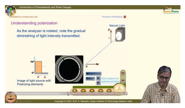
So, I should have two identical elements and put them crossed and gradually make them completely crossed, you find the intensity goes to zero. So, that indicates that what you have as shown is a polarized beam of light, which I have shown it for a white light now for a monochromatic light source.
