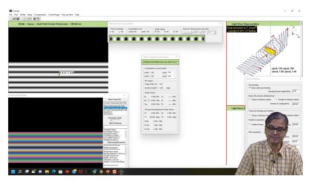
So, the intensity remains constant. And what you find here is, whenever I select a point here, when I get it very close to the actual fringe, you see the light is diminished. And you also see in this, what is the state of polarization as the light traverses the optical elements. So, you get a complete appreciation of what happens to the light at every stage. And you also have other facilities, because you have always seen fringes in color.
