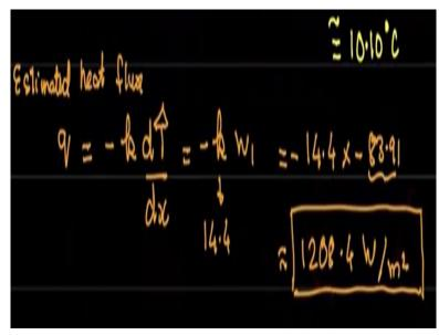
what is the estimated heat flux? So, the estimated heat flux q is,
