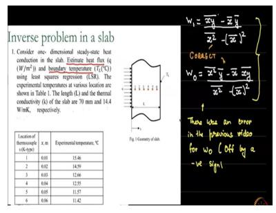
Welcome back. In the previous video we derived some simple expressions for linear model, recall that we were looking at the inverse problem in a slab. We have given thermocouple measurements at a few locations and we are asked to find out the actual temperature. So, what we are asked to estimate is that heat flux and the boundary temperature. So, we will try to answer this question, using the expressions that we derived in the last time.
