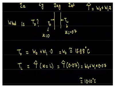
So, suppose I ask the question what is  $T_0$  that is the temperature on the left boundary? So, temperature at the right boundary now notice as far as the measurements are concerned. We do not have that value we only have thermocouple values in the middle of the slab 0.01 up to 0.06. we do not have a value at the left or the value at the right.
