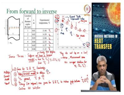
Now, here are the actual temperature measurements plotted. these are the x locations so this is i = 1, i = 2, etc., you can see that these are the temperature measurements. Notice that they do not lie on a line. as I told you with the ball falling through the air, in practice what you are going to see are you may call it noise, may be due to noise within the thermocouple, may be due to measurement error or maybe due to material in homogeneity.
