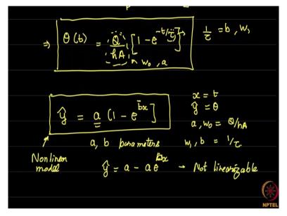
Now this forward model as if you can look at it basically has two parameters, it has this parameter  $\frac{Q}{hA}$  we can call this parameter as  $w_0$  or a. We have this other parameter  $\tau$  we can call  $\frac{1}{\tau}$  as b or  $w_1$ . So, in that case we can write this in the form,
