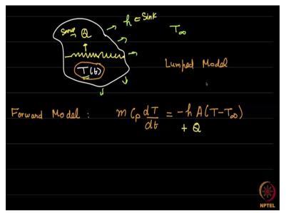
So, let me make up a simple lumped model of this, you can assume that this is somewhat like the chip and the fin system. It is kept at some constant temperature T so that is this temperature is especially constant wherever you keep a thermocouple roughly the same temperature is obtained. Of course, this depends on Biot number etcetera, which you would have seen in heat transfer since this is not a full course on heat transfer.
