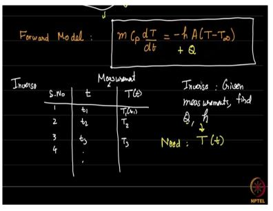
So, this model is a ODE as you can see, this is the temperature model. Now, what sort of inverse problem can we solve with this. So, the inverse problem could be something like this. Let us say we run an experiment and at various time points  $t_1$ ,  $t_2$ ,  $t_3$  so on and so forth. We actually measure the temperature kept at the body. So, you could have one single thermocouple or multiple thermocouples and find out an average temperature since we are taking a lumped model.
