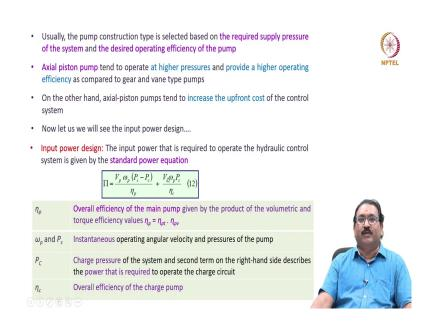
Usually, the pump construction type is selected based on the required supply pressure of the system and the desired operating efficiency of the pump. Axial-piston pump tend to operate at high pressures and provide a higher operating efficiency as compared to gear and a vane type pumps. On the other hand, axial-piston pumps tend to increase the upfront cost of the control system.
