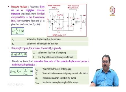
Pressure analysis, assuming there are no or negligible pressure transients that results from the fluid compressibility in the transmission lines. The volumetric flow rate Q A is given by already we know that Q A equal to AV - A into V. So, Q A equal to V a by nu a v into theta
