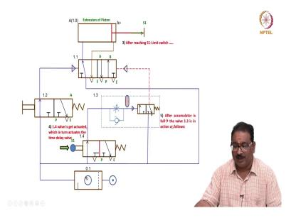
Now, how, what happens here? When after pressing this, the pneumatic energy will actuate the left position of the pilot operated valve. Then, air will come here enters the head side, start extending correct, it will start extending. After reaching this, what happen friends?
