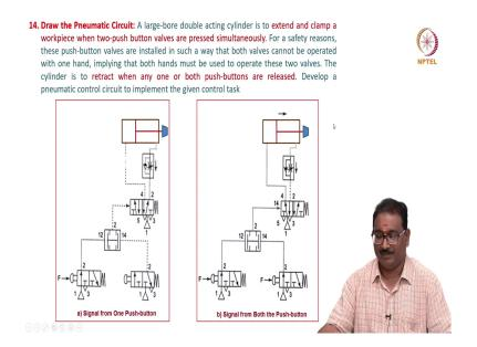
Now, 14th one. Draw the pneumatics circuit. A large-bore double acting cylinder is to extend and clamp a workpiece when two-push buttons are pressed simultaneously, then only it will work otherwise no. For a safety reasons, these push button valves are installed in such a way that both valves cannot be operated with one hand, implying that both hand must be used to operate these two valves.
