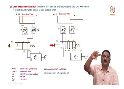
Next, draw the pneumatics circuit to control the forward and return speed of the double acting cylinder here, outflow is controlled. Show the power source and FRL unit. How to do here? Both forward and return should be controlled, but outflow is controlled. How to do? See here, the position of the check valve will matters.
