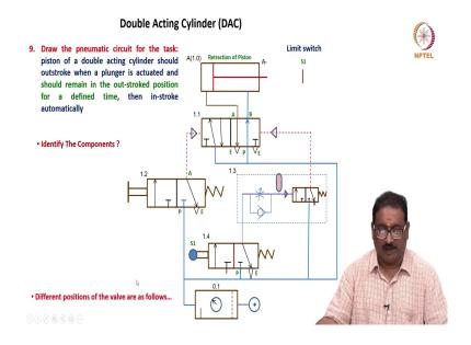
Now, we will see the 9th problem. Draw the pneumatic circuit for the task: the piston of a double acting cylinder should out-stroke when a plunger is actuated and should remain in the out-stroke position for a defined time, 10 second, 20 second, 30 second, you should wait because loading and unloading operation may takes place, then in stroke automatically, after waiting for a certain period. How to do this? Identify the components now.
