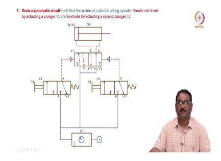
My name is Somashekhar, course faculty for this course. Next one, 7th problem. Draw a pneumatic circuit such that the piston of a double acting cylinder should out-stroke by actuating the plunger T1 and in-stroke by actuating the second plunger. Then you will see double acting cylinder put the pilot operated valve, one plunger another plunger, you will press it here, it will extend, press it again here, it will retract then power source we add it all.
