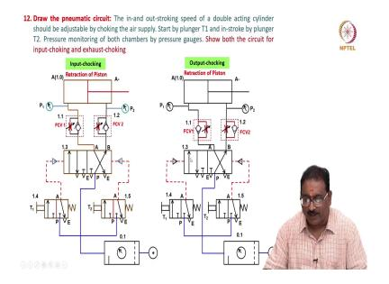
Now, we will see draw the next problem; next problem it is. Draw the pneumatic circuit. The in and out stroking speed of a double acting cylinder should be adjusted by choking the air supply. Choking means by controlling the air. Start by plunger T1 and in stroke by plunger T2.
