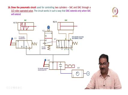
Now, I will show you one more circuit on this. Draw the pneumatic circuit used for controlling the two cylinders. Now, we will see single acting cylinder and a double acting
