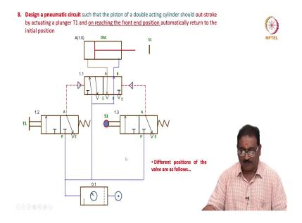
We will move on to the one more circuit, design a pneumatic circuit such that the piston of a double acting cylinder should out-stroke by actuating the plunger T1 and on reaching the front-end position, automatically returns to the initial position. Previously, you have to press T1 and T2, T1 for extension, T2 for retraction, now it is doing automatic operation. How will I achieve this? By putting the limits switch that is all, very very simple here.
