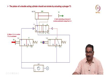
The piston of a double acting cylinder should out-strokes by actuating the plunger T1. Press it here, see here it will go here energy, it will actuates, extends correct it starts extending. After reaching this, what happen? See here, after reaching this, the energy will come here, actuate this position.
