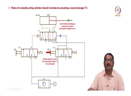
Then, piston of a double acting cylinder should in stroke by actuating this. Press again one more, it will go to here, no signal here. When you will press this here, the pneumatic energy will come here, actuate this position. What happened? The air will enters to the tail side, then it is pushing, air will go to the atmosphere through this port. Meaning, it will retract through plunger T2 extension through T1, retraction through T2.
