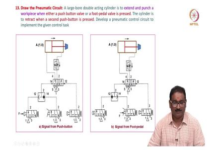
Now, we will move on to the 13th circuit. Draw the pneumatic circuit. A large-bore double acting cylinder is to extend and push a workpiece when either a push button valve or a foot-pedal valve is pressed. Any one is pressed, it should out stroke. The cylinder is to retract when a second push button is pressed. Develop a pneumatic circuit to implement the given control task. How to do this? You will see, now I am using the shuttle valve here.
