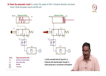
10th problem. Draw the pneumatic circuit to control the speed of single acting cylinder in forward direction and quickly return. Show the power source and FRL unit. Very simple here, we have seen these type of problems in the hydraulics also same thing here, I am putting the 1.2 is a work flow controlled valves, again it is a single acting cylinder it controlled through the 3 by 2 DCV power source.
