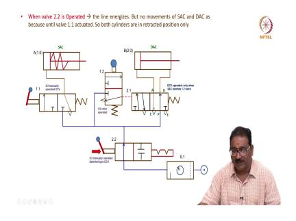
When the valve 2.2 is operated, the line energizes, main valve is there know 2 by 2 valve. But no movements of SAC and DAC as because until the valve 1.1 actuated. So, both cylinders are in the retracted position only where it is this is 2 by 2 manually operated detented type DCV, always you have to use this friends because either it will sends the flow or blocks the flow, then only line will energize, always it is a main control here whole circuit.
