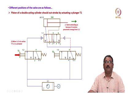
How it will operate? I will show you the position, different position. When you will piston of a double acting cylinder should out-stroke by actuating the plunger T1. If you will press this, what happen? You will see here the signal will come here. Then, what happened? The energy will come here, come here, enters to the head side, it will extend, start extending because it receives the pneumatic energy from the 1.1.
