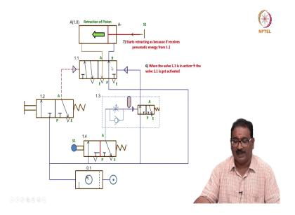
Then, it starts retracting because as because it receives the pneumatic energy from 1.1 because it is actuated. When the 1.3 is in action, the valve 1.1 get actuates, then it will return simple, very simple.
