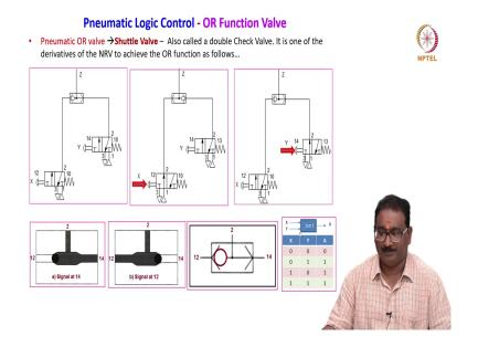
Then, I will show you some more valves. Pneumatic logic control, we are using the OR function valve. You already studied this OR gates in the digital electronics; same way here, the pneumatic valves are there. The pneumatic OR valve, it is known as a shuttle valve, also called a double check valve.
