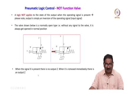
Move on to the pneumatic logic control, here NOT function valve. A logic NOT applies to the state of the output when the operating signal is present. Please note the output is simply an inversion of the operating signal that is a input signal, it is an inversion. The valve shown below is normally open type that is without any signal to the valve, it is always get opened in the normal position.
