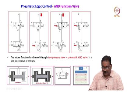
Now, we will move on to the pneumatic logic control the AND function valves. You will see here how it will work. The Z is an output whatever it is, now always you have to draw the signal in the outlet positions correct. When I will get the Z, when you will press this, what happen? Here it will come, but again it is locked position.
