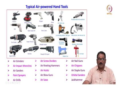
Typically, air powered hand tools are numerous use in industry. Some of them are I am listing here; they are the air grinders, air impact wrenches, air sanders, paint sprayers, air drills, air screw drivers, air riveting hammers, air hoists, air blow guns, air saws, air nail guns, air chippers, air staple guns, orbital sanders, jackhammers. The many tools are there, these are known as typical air-powered hand tools. They will use the compressed air for their operations.
