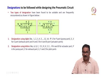
Then, quickly, we will see the designations to be followed, while designing the pneumatic circuits. Two types of designations have been found to be suitable and are frequently, encountered as shown in the figure below. You will see there are two types of designations for the valves, actuators all.
