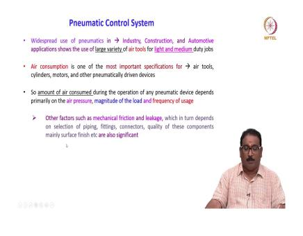
Widespread use of pneumatics in industry, construction, automotive applications shows the use of large variety of air tools for light and medium duty jobs. Air consumption is one of the most important specifications for air tools, cylinders, motors and other pneumatically driven devices.
