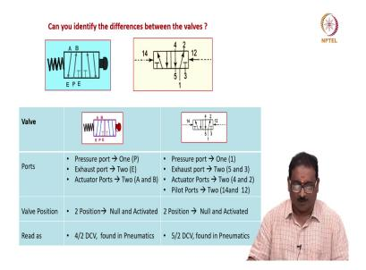
Next, we will move on to the one more valve, can you please identify the difference between these two, as I already shown you in the previous slide. Quickly, we will see the number of ports, all these thing. Number of ports, the pressure port is there; correct friends? Exhaust port, 2 exhaust port and actuator ports A and B.
