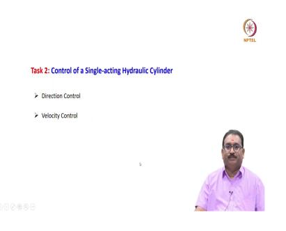
Now, I will show you some other circuits which are very essential to understand when we are operating the different types of actuators. Now, let us we will see the task 2: control of a single acting hydraulic cylinder, single acting hydraulic cylinder, meaning single port is there that is head side or a tail side. But, now I am taking the head side is a input port meaning the pressurized fluid is taken and acting on the complete piston area then it will extend.
