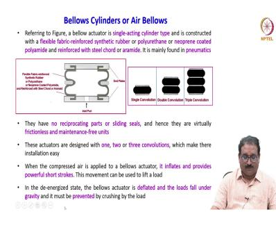
Now, we will see one more type bellow cylinder also known as air bellows. Referring to the figure, a bellow actuator again here it is a single-acting cylinder type and is constructed with the flexible fabric-reinforced synthetic rubber or a polyurethane or a neoprene coated with polyamide and reinforced with steel chord or a aramide.
