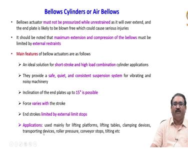
Bellow actuators must not be pressurized while unrestrained as it will over extent and the end plates is likely to be blown free which could cause a serious injuries. It should be noted that maximum extension and a compression of the bellows must be limited by external restraints. Main features of the bellow actuators are as follows.
