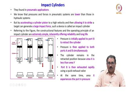
Then we will see the impact cylinders. Again they have found wide applications in pneumatics. We know that the pressures and forces in pneumatic systems are lower than in hydraulic systems. But by accelerating the cylinder piston to a very high velocity and then allowing it to strike a target can generate a larger impact force, such a device is called a impact cylinder.
