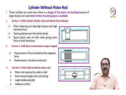
Now we will see quickly the cylinder without the piston rod previously the piston rod where the load is attaching it will do the extension interaction of the load for positioning applications or many applications, but here now there is no piston rods. Then you will see the different versions available in this category.
