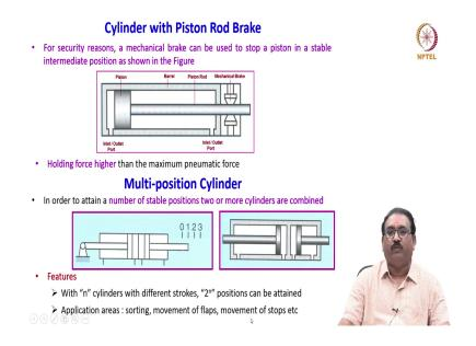
Now, we will see some more types cylinder with piston rod brake. For security reasons, a mechanical brake can be used to stop a piston in a stable intermediate position as shown in the figure here. Here you will see it is a similarly it is a double acting cylinder, but an arrangement is made for breaking the piston rod during the motion.
