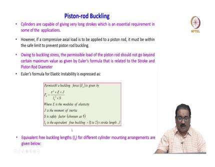
As I have told you cylinders are capable of giving a very long strokes which is an essential requirement in some of the applications. However, if the compressive axial load is to be applied to the piston rod, it must be within the safe limit to prevent the piston rod buckling.
