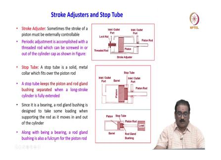
My name is Somashekhar, course faculty for this course. Then we will see some more arrangements are there in the cylinders the Stroke adjusters and Stop tube. What is this stroke adjuster? Sometimes the stroke of a piston must be externally controlled. You will see here this is a threaded rod, lock nut, inlet outlet port, this is a barrel, inlet outlet port piston with seals and you will see here this can be moved in and out with a threaded rod with lock nut.
