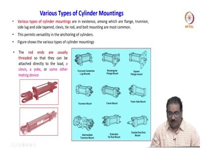
The various types of cylinder mountings are in existence among which are a flange, trunnion, side lug and a side tapered, clevis, tie rod and a bolt mounting are most common. I will show you some of the cylinder mounting here these are permits the versatility in the anchoring of the cylinders.
