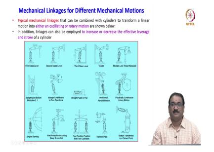
Then we will discuss some of the mechanical linkages for different mechanical motions. Typical mechanical linkages that can be combined with cylinders to transfer a linear motion into either an oscillatory or rotary motion as shown in the figure below. In addition, the linkages can also be employed to increase or decrease the effective leverage and a stroke of the cylinder.
