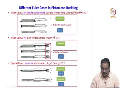
You will see the different cases are there for the mounting, the Euler case 1 here you will see the ends of the rod is free lateral. For a slender column with one end free and the other end fixed, 1 k free buckling length 1 k equal to 2 into 1, 1 is a stroke complete stroke. Euler case 1 1 k equal to 2 l.
