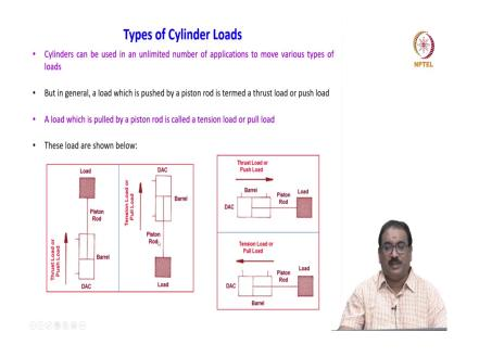
Now, quickly we will see the different types of cylinder loads. Cylinders can be used in an unlimited number of application to move the various types of loads. But in general, a load which is pushed by the piston rod is termed as a thrust load or a push load. A load which is pulled by a piston rod is called a tension load or a pull load. You will see the cylinder load
