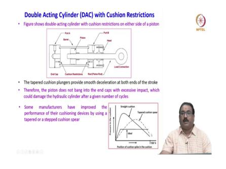
Now, I will show you the double-acting cylinder with a cushion restrictions on either side. You will see here the cushion restriction arrangements what they made here, cushion restriction arrangements what they made in the two end caps, end cap here and the rod end cap how they made the arrangement, ok. Here it will enters.
