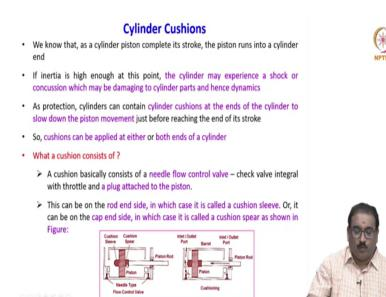
Now, we will see friends the cylinder cushions are playing a major role to overcome the impact of the piston when it reaches the two extreme ends. What are these? We know that as the cylinder piston completes its stroke, the piston runs into the cylinder end. If the inertia is high enough at this point the cylinder may experience a shock or a concussion which may be damaging the to the cylinder parts and hence effects the dynamics also.
