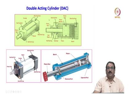
Now, we will see this the constructional details of double-acting cylinder single rod. See here friends how it looks, three-dimensional things I have shown you here. The schematic diagram as well as the actual double-acting cylinder it is a cut section model here. Here it is a piston rod, piston rod, which will carries the load here, correct.
