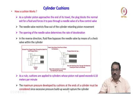
Let us we will see this also. I will explain to with figure. Same figure it is here. Here I am showing you the one side cushion spear, how it will work. As a cylinder piston approaches the end of its travel, the plug blocks the normal exist for a fluid and forces it to pass through the needle valve of the flow control.
