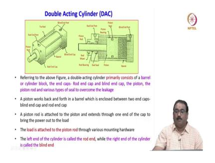
Now, let us we will see very quickly referring to the above figure, a double-acting cylinder primarily consists of a barrel or a cylinder block, the end caps; rod end cap and a blind end cap, the piston, the piston rod and a various types of seals to overcome the leakage.
