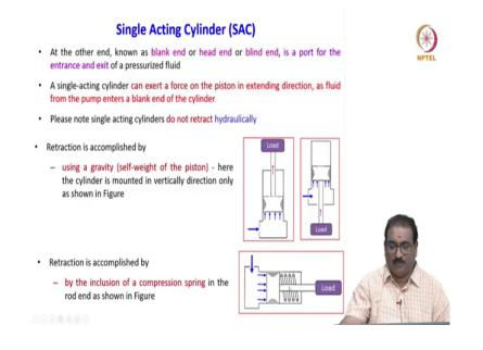
At the other end known as a blank end, also known as head end or a blind end is a port for the entrance and exit of the pressurized fluids. A single acting cylinder can exert a force on the
