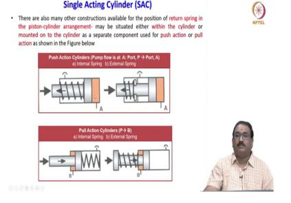
Now, we will see there are also the many other constructions available for the position of the return spring in the piston cylinder arrangement, may be situated either within the cylinder as you have seen, or mounted on to the cylinder as a separate component used for push action or a pull action as shown in the figure here. This is based on the how the stiff spring is placed, you will see now here. Here the push action.
