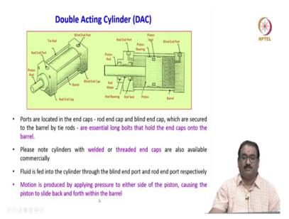
What are these tie rods? Are essentially the long bolts that hold the end caps on to the barrel. Please note friends, cylinders with welded or a threaded end caps are also commercially available. Do not think always that the tie rods they are using, need not necessary.
