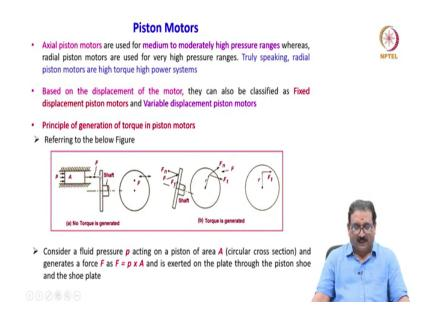
Axial piston motors are used for medium to moderately high pressure ranges, whereas, radial piston motors are used for very high pressure ranges. Truly speaking, radial piston motors are
