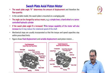
The swash plate angle theta determines the amount of displacement and therefore, the quantity of fluid. In the variable model, the swash plate is mounted on a swinging yoke. The angle can be changed by the various means, that is use a simple lever, or a hand wheel, or a servo controlled hydraulic cylinders.
