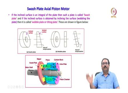
If the inclined surface is an integral of the plate, then such a plate is called a swash plate. And if the inclined surface is obtained by inclining the surface meaning by wobbling the plate that
