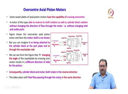
Then some of the cases, the over centre axial piston motors serves the many purpose. What are those? We will see now. Some swash plates of the axial piston motors have the capability of crossing over centre. A motor of this type able to reverse its shaft rotation as well as a cylinder block rotation without changing the direction of flow through the motor that is without changing the fluid flow in the inlet and outlet ports.
