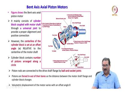
Now, we will see the one by one how the constructional features and generation of torque in each type of motor. First one is bent-axis axial piston motor. The name itself tells us that the cylinder block and the motor shaft, here what I am written here a drive shaft inclined to each other.
