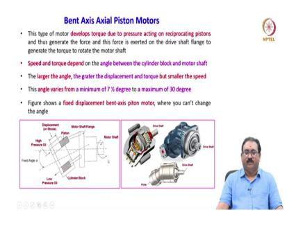
This type of motor develops a torque due to pressure acting on reciprocating pistons and thus generate the force and this force is exerted on the drive shaft flange to generate the torque to rotate the motor shaft. Speed and torque depend on the angle between the cylinder block and motor shaft.
