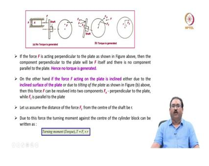
If the F is acting perpendicular to the plate as shown in the figure here, then the component perpendicular to the plate will be F itself, and there is no component parallel to the plate. Hence, no torque is generated. When it is? When the forces acting perpendicular to the flange of the shaft.
