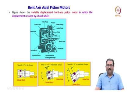
Here you will see the figure shows the variable displacement bent-axis piston motor in which the displacement is varied by a hand wheel, the hand wheel is provided and then yoke is there, correct. You will rotate the hand wheel for adjusting the theta. When theta is 0, meaning when the cylinder block is aligned with the motor shaft, no stroke; pistons are on the same line that is why there is no torque.
