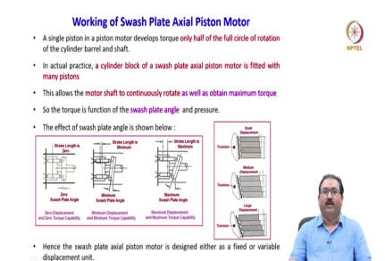
A single piston in a piston motor develops a torque only half of the full circle rotation of the cylinder barrel and a shaft. In actual practice, a cylinder block of a swash plate axial piston motor is fitted with the many pistons. Generally for the smooth operation, they are odd in numbers; 7, 9, 11 like this which will provides the pressure is meaning smooth pulsation.
