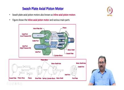
Now, we will move onto the swash plate axial piston motor. Swash plate axial piston motors are also known as inline axial piston motors. See here the figure shows the inline axial piston motor at a various parts. You will see here friends the inlet port is there, meaning high pressure oil from the pump and control elements will enter here. These are the pistons.
