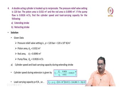
A double acting cylinder is hooked up to reciprocate the pressure relief valve setting is 120 bar. The piston area is 0.032 metre square and the rod area is 0.0090 metre square. If the pump flow is 0.0026 m cube per second, find the cylinder speed and load carrying capacity for the following meaning for extending stroke as well as retracting stroke.
