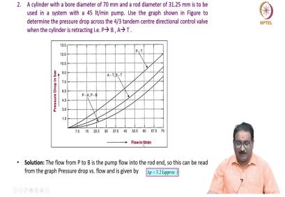
I will show you one more. A cylinder with a bore diameter of 70 mm and a rod diameter of 31.25 is to be used in a system with a 45 litres per minute pump, use the graph. Here the graph is given in the figure which will shows the pressure drop across the flow in litres per minute.
