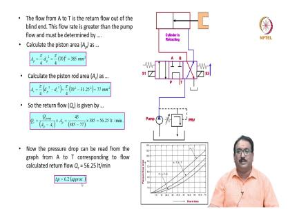
Next, this is a configuration as I have to P to T, A to B, now they are asking for the crossed configuration. They may asked for this also. Now we will see the pump flow is connecting to the tail side or a rod side, the head side is connecting to the tank. So, the flow from the see here A to T how it is A to T is the return flow out of the blind and this flow rate is greater than the pump flow, correct?
