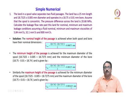
My name is Somashekhar, course faculty for this course, correct friends? Now, I will solve some of the simple numerical problems for the directional control valve, pressure control valves and a flow control valves very quickly. The problem is like this. The land in a spool valve separates two fluid passages.
