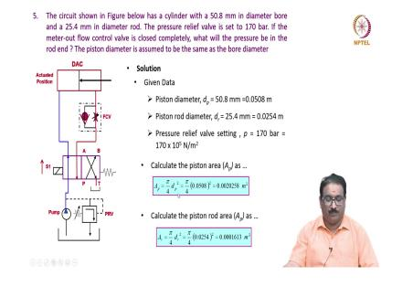
5th problem; the circuit shown in figure below has a cylinder with 50.8 mm in diameter bore and a 25.4 mm in diameter rod. The pressure relief valve setting is 170 bar. If the metre out circuit because you will see here metre outflow is controlled metre outflow control valve is closed completely, you will see here if the metre out flow control valve is closed completely what will be the pressure be in the rod end? The piston diameter is assumed to be the same as a bore diameter.
