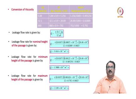
So, now viscosity as I have told you it is given in the cSt kinematic viscosity and converting into centipoise by multiplying with the specific gravity of the fluid assumed to be 0.9. I am converted here, then I am converting in to SI unit Newton second per metre square; Newton per metre square is a Pascal and second is a s. I am writing here Pascal second and converted here, how to convert? After getting this divided by 1000s.
