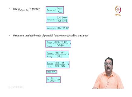
Now, the pressure when full pump flow which is given by F force by an area fully open and poppet substituting the value here, then after simplification what I will get here? 762 l plus
