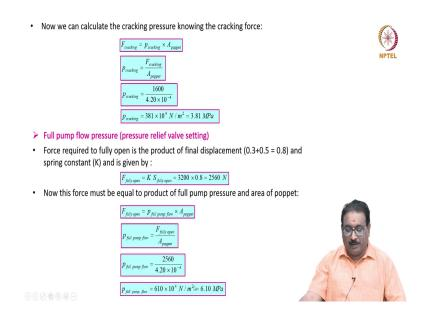
Now, we can calculate the cracking pressure knowing the cracking force; the F cracking equal to P cracking into a poppet area of the poppet. So, P cracking equal to F cracking divided by a poppet. Now, we will substitute the value 1600 area of the poppet is given, but please take care friends all unit should be in the same unit, all centimetre I am converting into the metre. Now, we will get here Newton per metre square, then it is nothing but 3.81 mega Pascal.
