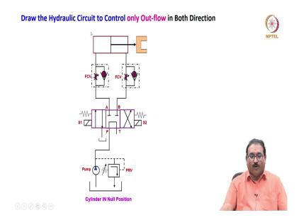
Now, similarly you will see here draw the hydraulic circuit to control only the outflow in both direction, see the position of the check valve very important here friends, because how we are connecting that will matters always as usually you have to draw the circuit in the null positions; again it is a tandem neutral correct the pump PRV all are same S 1 and S 2 are solenoid actuator valve.
