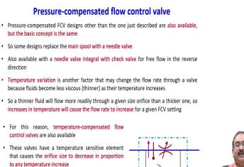
• Fig shows the graphic symbol for pressure-andtemperature compensated FCV with check valve
