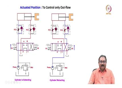
Now we will see in the when S 1 is operated, what which flow is controlled you will see now; pump flow is coming here, then you will see now friends here it will not pass through the opened orifice, it will bypass because the ball will lifted up from the valve seat, it will enters here flow is not controlled. Then from the rod side flow will come here it will pass through the metered orifice.
