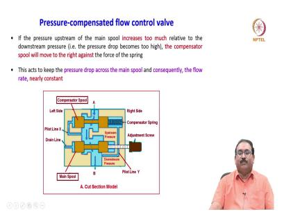
If the pressure upstream you will see the pressure upstream of the main spool increases too much relative to the downstream pressure; meaning, the pressure drop becomes too high the compensator spool will move to the right side against the force of the spring.
