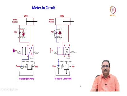
Let us will see how this circuits will looks, this is a metering circuit what I have drawn here, here is the Double Acting Cylinder DAC first one is a normal position meaning always the circuit you have to draw only in the retracted position meaning it is a normal position. Here as usual the 4 by 2 DCV solenoid actuation springs center, here you will see the flow control valve what I have drawn here.
