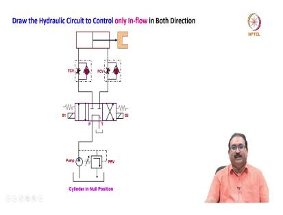
Now, we will see draw the hydraulic circuit to control only inflow in both directions, you will see now inflow in both direction; now only way is I am using the flow control valve head side as well as a tail side. Now we will see always you will draw the circuit in the null position
