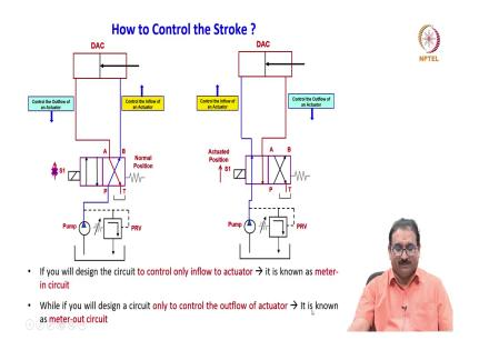
Now, quickly we will see the application of these flow control valves; How to control the stroke here? Now we will see this here this is a Double Acting Cylinder DAC connected to
