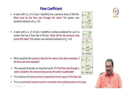
Quickly I will show you the significance of the flow coefficient. A value with a C v of 2.5 lpm per square root of k Pascal has a pressure drop of 200 kPa kilo Pascal. What must be the flow rate through the valve? The system uses a standard hydraulic oil S g equal to 0.9. Very quickly Q equal to already we know that C v into root delta P by S g substitute the given value.
