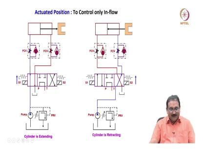
Let us will see here if the S1 is operated what happens? You will see the pump flow is coming here and it will not pass through the check valve, because position you will see here only it will pass through the orifice how much you are opened meaning the inflow is controlled. Then whatever the flow is there at the rod side it will bypass through the check valve meaning inflow is controlled when S1 is operated.
