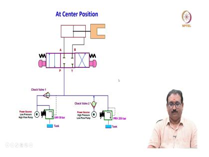
Here I am setting the pressure 250 bar. Then both are connected to the tank. Please note friends. Then we will see what happens, when I push this button, and what happens if I will push this button? Then what is the role of these two relief valve setting? We will see now. At center position, center position, no need to worry friends correct. All the flow will come here accumulate here, correct.
