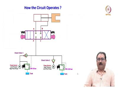
After knowing this, now I will explain to you, this unloading valve in one particular application which is used to control the double acting cylinder. This is a double acting cylinder connected to the 4 by 3 direction control valve, closed center push button actuation, spring centered. And this is connected to the power source 1 – here low pressure high flow pump; and one more is the high pressure low flow pump.
