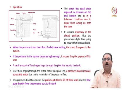
The piston has equal areas. Here you will see this area and this area full exposed meaning on the top side and a bottom side, the pressure going to the system is acting here.
