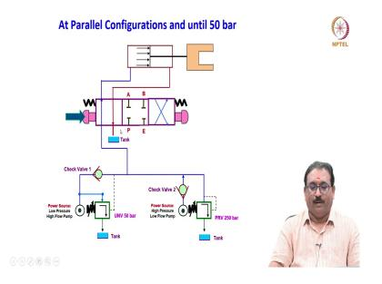
Until how many bar? Until 50 bar, because I have set the 50 bar setting here. After reaching the 50 bar setting, what happen? Automatically this will open. Then whatever the flow is coming from low pressure high flow pump will go into the tank. Only actuator after reaching, it will receives the flow from the high pressure low flow pump, then it will move very slowly as compared to previous one. Until how much it is? Until it is the pressure setting of 250 bar.
