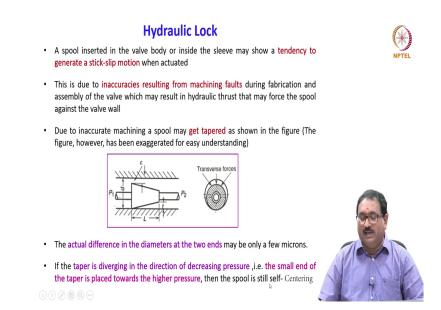
Next important parameter, one more you come across is a hydraulic lock. What is this, what are the causes for it? A spool inserted in the valve body or inside the sleeve may show a tendency to generate a stick slip motion when actuated. This is due to inaccuracies resulting from the machining faults during fabrication and assembly of the valve which may result in hydraulic thrust that may force the spool against the valve.
