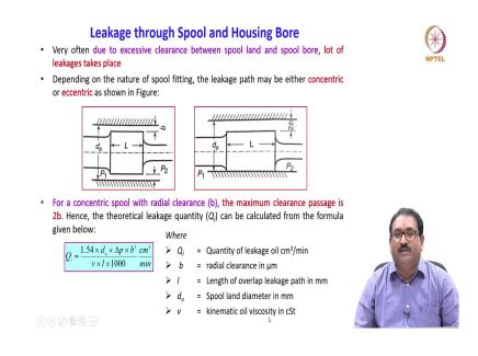
Now, we will see the leakage through the spool and housing bore. Quickly you will see. [FL] Very often due to excessive clearance between the spool land and a spool bore, a lot of leakage takes place. Depending on the nature of the spool fitting, the leakage path may be either concentric or eccentric as shown in the figure here.
