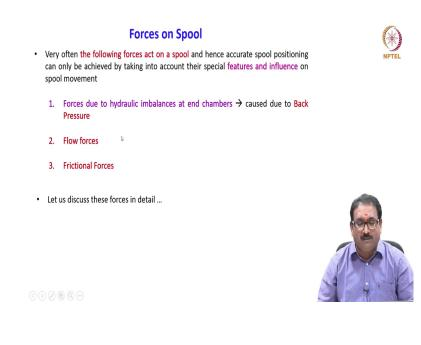
Quickly we will see the sum of the forces on spool. Very often the following forces act on the spool and hence accurate spool positioning can only be achieved by taking into account their spatial futures and influence on the spool movement. First one; forces due to hydraulic imbalance at end chambers caused due to back pressure, flow forces, frictional forces.
