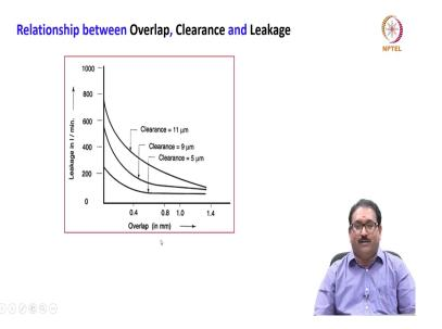
Now, we will see the relationship between the overlap, clearance and a leakage. That this clearance is the distance between the spool and the valve body, meaning diametrical clearance it is. You will see here; the I have drawn the plot here leakage versus the overlap.
