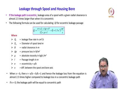
If the leakage path is eccentric, as I have shown you in the previous slide, leakage area of the spool with a given radial clearance is almost 2.5 times larger than when it is concentric. The following formula can be used for calculating the leakage Q l for the eccentric type. Q l equal to pi d o into delta p b cube by 12 mu l into 1 plus 1.5 e cube centimeter cube per second, provided you will use all the quantities in the same units.
