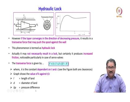
However, if the taper converges in the direction of decreasing pressure, it results in transverse force that may push the spool against the wall. This phenomenon is termed as hydraulic lock. Actually, it may not necessarily result in a lock, but certainly it produces a increased friction and noticeable particularly in case of servo-valves.
