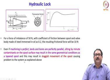
For a force of imbalance of 50 Newton, with a coefficient of friction between the spool and valve body made of steel immersed in oil as 0.2, the resulting frictional force will be 10 Newton.
