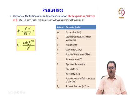
Very often the friction value is dependent on factors like temperature, velocity of air etcetera. In such cases the pressure drop follows the empirical relation is delta p equal to beta by RT v square by d l p. Again, here you will see friends delta p you will get it in bar provided the beta is the coefficient of resistance which varies with G. What is a G? G is a friction factor is determined using 1.6 Q a raised to 1.85 divided by d to the power of 5.
