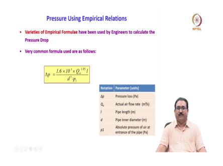
Varieties of empirical formulae have been used by engineers to calculate the pressure. Very common formula is delta p equal to 1.6 into 10 to the power of 3 into Q a raised to 1.85 into 1 divided by d to the power of 5 into p 1.
