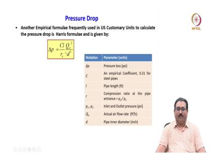
Another empirical formulae frequently used in US Customary Units to calculate the pressure drop is a Harris formulae more frequently used in US and is given by delta p equal to Cl by r c Q a by d here 2 and here 5. You will see what is delta p; you will get it in the psi pounds per square inch US Customary Unit.
