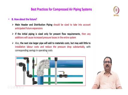
Then how about the future? Main header and distribution piping should be sized to take into account anticipated future expansions. If the initial piping is sized only for present flow requirements, then any additions will cause increased pressure losses in the entire system. Also, the next size larger pipe will add to material costs, but may add little to installation labour costs and reduce the pressure drop substantially, with corresponding saving in the operating cost.
