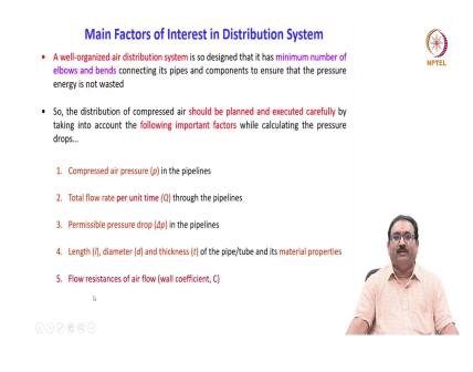
Now, quickly we will see the main factors of interest in distribution system. A well-organized air distribution system is so designed that it has a minimum number of elbows and bends, correct friends? Connecting it is pipes and a components to ensure that the pressure energy is not wasted.
