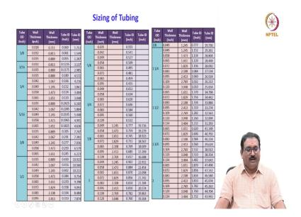
Here I am showing you the different types of tube OD wall thicknesses. Tube OD it is 1 by 8th inch, 3 by 16th, 1 by 4 different tube OD and corresponding wall thicknesses in inch millimeter. Similarly, tube ID and tube ID inch and millimeter; this these are all you will get all this information in the pneumatic manuals based on your requirement you will choose the required OD and corresponding wall thicknesses.
