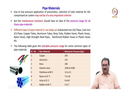
Then, materials for the pipe as well as the tubes. Due to low pressure application of pneumatics as I have told you 6 to 10 bar is a normal pneumatics the people will never go beyond 20 bar. So, due to low pressure application of pneumatics selection of tube material for compressed air system may not be of very important criteria.
