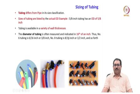
Then you will see sizing of the tubes the tube differs from pipe in it is size classification. Sizing of pipes is different, sizing of tubes are different. Here in sizing of tubes are listed by the actual OD example 5 by 8 inch tubing has an OD of 5 by 8 inch.
