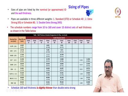
Let us we will see sizing of pipes. Sizing of pipes are listed by the nominal or approximate ID inside diameter and the wall thickness. Pipes are available in 3 different weights, what we
