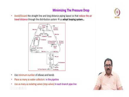
Also avoid or discard the straight line piping and tubing and long distance piping avoided, so that reduces the air travel distance through the distribution system. That is why I am telling you always adopt the looping system. You already know what is a looping system.
