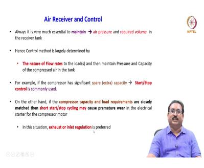
Air receiver and a control always it is very much essential to maintain the air pressure and a required volume in the receiver tank. Hence control method is largely determined by the nature of the flow rates to the loads and then maintain the pressure and capacity of the compressed air in the tank.
