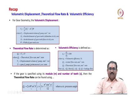
Let us we will see now friends how to ascertain this. Already, we have seen for the given gear geometry the volumetric displacement per revolution, how much oil it will discharge? This is a area multiplied by the width of the gear pi by 4 D o square minus D i square into W.
