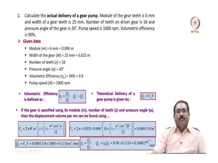
Move on to the next problem, calculate the actual delivery of the gear pump. Module of the gear is 6 mm and width of the gear is 25 mm. Number of teeth on the driver gear is 18 and pressure angle of the gear is 20 degree. The pump speed is 1000 rpm. Volumetric efficiency
