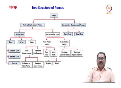
Also, we have seen the tree structure of the pump quickly. Pumps positive and non-positive, we discussed in the last class. Here, we concentrated more on rotary pumps in which gear pump, screw pump; external gear pump; internal gear pump; gerotor. In this category, it is a rotary action; but here along the axis, the fluid will be transported.
