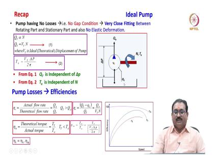
Also, we discussed the ideal pump. What is ideal pump? Pump having no losses. What is the meaning? No gap condition; meaning, very close fitting between the rotating part and the stationary parts and also, no elastic deformation. Please note friends, this is to arrive the some
