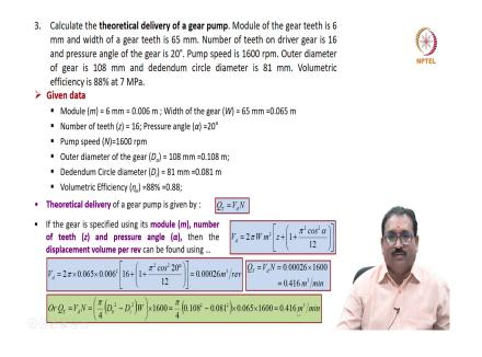
Let us we will see one more problem. Calculate the theoretical delivery of a gear pump. Module of the gear teeth is 6 mm and width of the gear is 65 mm. Number of teeth on driver gear is 16 and a pressure angle of the gear is 20 degree. The pump speed is 1600 rpm. Outer diameter of gear is 108 mm, dedendum circle diameter is 81 mm. Volumetric efficiency is 88 percent at 7 MPa.
