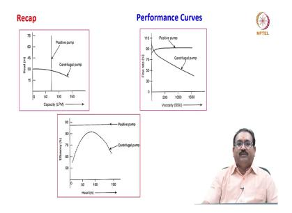
Later, we have seen the some of the characteristics about the positive displacement pump and non-positive displacement pump like a centrifugal pumps. The head versus capacity, you will see the positive displacement remains same; but centrifugal pump, it will goes on decreasing.
