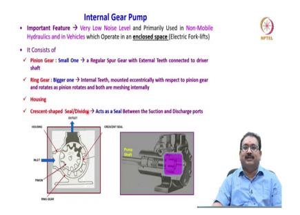
So, important features are here, very low noise level and primarily used in non mobile hydraulics, and in vehicles which operate in an enclosed space like a electric forklifts. It consists of, you will see here I have shown the sketch again here; you will see here driver and
