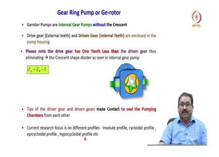
What is this? Gerotor pumps are a again a internal gear pumps without the crescent shaped divider. You will see here, the driver gear, meaning the driver external teeth; meaning is a pinion it is, remember external teeth, external teeth and a driven gear internal teeth with what we will call bigger gear are enclosed in the pump housing.
