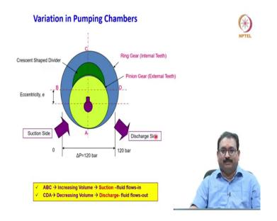
Then, I will quickly I will show you this variation in the pumping chamber with simples schematic diagram; you will see here friends as I have told you, the ring gear is a big one and axis is here I marked and it is see here pinion gear which has a external teeth mounted eccentrically.
