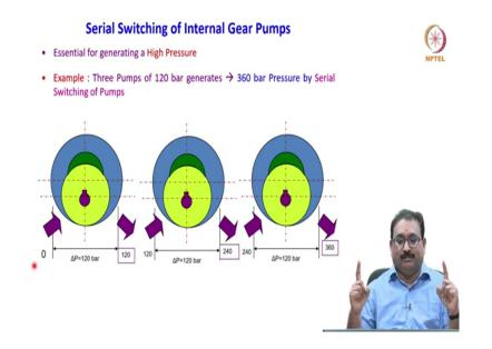
Now, very very important thing in the internal gear pump is serial switching of the internal gear pump is possible. For example, look here as I have told you in the previous slide, the pump is designed for the certain pressure; for example, delta P is 120 bar. You cannot use this pump beyond 120 bar; otherwise the pump elements will get destroyed or what happens the pump efficiency will go off for the continuous usage.
