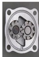
Cut section of a External Gear Pump
