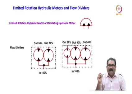
Now, we will move on to limited rotation hydraulic motors and flow dividers we will see now how to represent; limited rotation friends, how to represent? Semi circle with a triangle two triangle filled it is read as, limited rotation hydraulic motor are also known as oscillating hydraulic motor meaning, semi circle. Flow dividers, what are these flow dividers friends?
