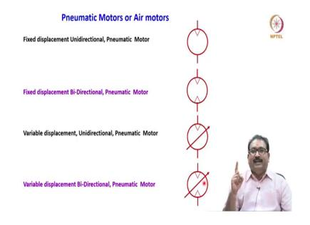
Later we will move on to now the pneumatic motors are also known as air motors, how to represent? See same previously correct, but triangle is not filled, how to read? Fixed displacement unidirectional, pneumatic motor; if we will put two arrows here triangle not filled it is read as a fixed displacement bidirectional, pneumatic motor.
