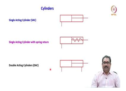
Later we will move on to the cylinders; cylinders again actuator they will convert the fluid energy into the mechanical as a force and velocity linear velocity here. Let us we will see how to represent the cylinders. Single acting cylinder, see friends one rectangle then one line and big line, please see here I am putting one line here, what is this? What is the meaning of this?
