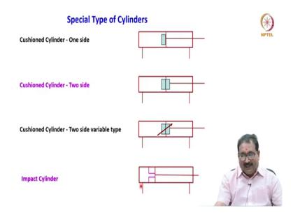
The special type of cylinders are there more frequently used, what are those? Cushioned cylinder one side, cushioning action is there they will put one pad here cushioned cylinder it is. How they will operate we will see later, but we will understand. Cushioned cylinder two side two pads they will put here or both are double acting cylinder remember here double acting cylinder, but cushion is there single side and two side.
