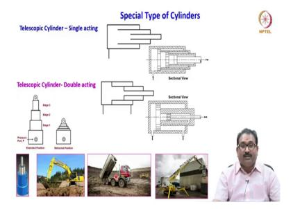
Now, we will move on to the telescopic cylinders it is a single acting you will see. What is telescopic cylinder? You will see the sectional views one tube inside the other, how the extension will takes place? Using the fluid energy; only one I will put single acting, if you will put two here extension and retraction of these tubes inside is through the fluid energy, you will see the sectional views and a fluid power symbol here.
