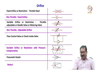
Then I will tell you the Orifice; what for orifice? To control the flow rate to the hydraulic systems or a pneumatic systems whatever it is. Now, we will see this the fixed orifice or a restriction meaning, throttle fixed they are represented like this. See the fixed restriction or a orifice, then a disc throttle they represented like this understand the symbol.
