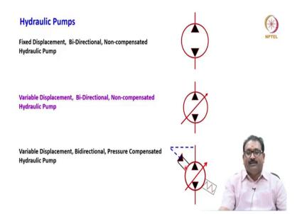
Then you will see here also we will see here 2 arrows I filled here. How we will read it? Fixed displacement, bidirectional, non pressure compensated hydraulic pump. The variable displacement, bidirectional, non pressure compensated hydraulic pump arrow same here variable displacement, bidirectional; then variable displacement, bidirectional, pressure compensated hydraulic pump see here same here, but you have to make the connections here.
