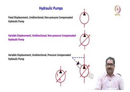
Now, we will move on to the hydraulic pumps. Already we know that the hydraulic pumps sucks the fluid from the tank and delivers to the rest of the system. Meaning, it will convert the mechanical energy received from the electric motor into the hydraulic energy.
