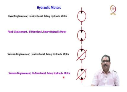
Now, we will move on to the hydraulic motors, what are these? Hydraulic motors are the actuators which will use the hydraulic energy to mechanical motions, like a force or a velocity here the hydraulic motor, what is very important here? It will gives the torque and the speed the actuators will convert the fluid energy into the mechanical parameters.
