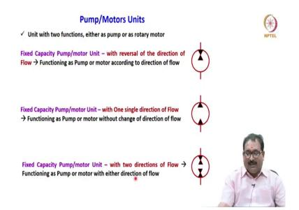
Later we will move on to the pump bar motor units you will see pump bar motor units. It is a unit with two functions, either as a pump or as a rotary motor depending on the flow that is why I am telling you. You will see here; see here friends how they are representing one arrow towards center another arrow towards out, again it is having inlet and outlet, how to read.
