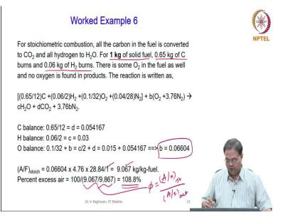
Now, what is asked here is the actual air supplied and percentage excess air; that means, you have to calculate what is the stoichiometric air. For stoichiometric combustion all the carbon in the fuel is converted into  $CO_2$  all hydrogen into  $H_2O$ .
