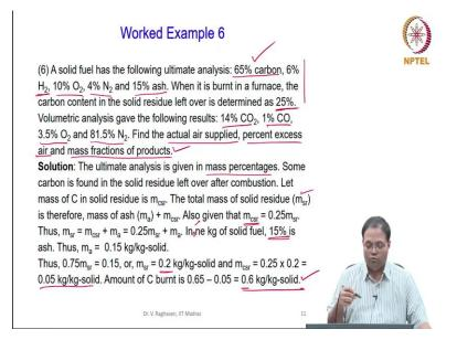
Now, worked example 6. We have dealt with the liquid fuel gaseous fuel etcetera. Now, we will go to a solid fuel, ok. Understanding a solid fuel let us say coal or something which has the following ultimate analysis. Ultimate analysis normally gives the elements which is present in the coal.
