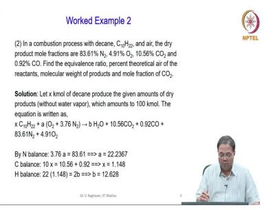
Second problem, we measured the exhaust dry fractions of the products, excluding the water vapour, and when you burn decane we got the product composition basically. (Refer Slide Time: 05:58)
