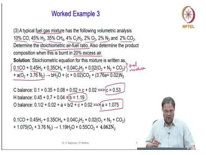
Third problem was a fuel mixture. Gaseous fuel mixture CO,  $H_2$ ,  $CH_4$ ,  $C_2H_2$  in some proportions are given. We need to determine the stoichiometric air fuel ratio and a product composition when it is burnt in excess air. That we did here.
