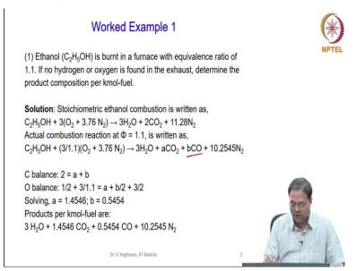
So, first we saw the problem with ethanol in a rich mixture 1.1 equivalence ratio and we saw that the hydrogen fully burns and carbon dioxide is not fully formed. Some amount of CO was present and we got the product composition.
