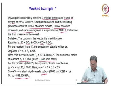
So, this is the last example. Here you can see that a rigid vessel initially contains 2 kilo moles of carbon. Carbon is in solid phase and 2 kilo moles of oxygen at standard temperature of 25°C and, but pressure is 200 kilo Pascals, combustion occurs.
