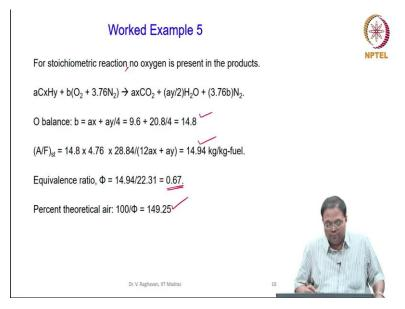
Now, this is the actual reaction where you have excess oxygen in the product. For stoichiometric reaction, no oxygen is present in the products. Again, we can put the same equation.
