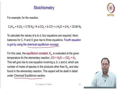
That is what I have explained here, to calculate the values of a to d, four equations are required. Atom balance C, H, O gives three equations and the fourth equation is got by chemical equilibrium. Now, for this particular case we can use this equation. I have shown three elementary equations in the in this slide;  $CO_2 \rightarrow CO + (1/2) O_2$ ,  $H_2O \rightarrow H_2 + (1/2) O_2$ .
