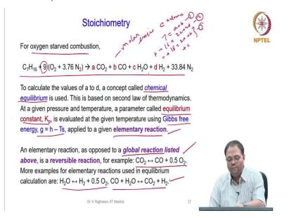
Again I am taking the same equation for oxygen starved combustion, you see that we have to use what is called as concept of chemical equilibrium; which is dependent on the second law of thermodynamics. What I am saying is we do not have sufficient data to analyze this.
