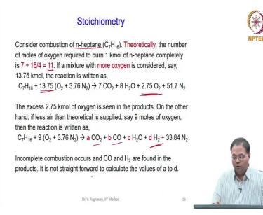
Now, let us consider n-heptane as a fuel  $C_7H_{16}$ . Theoretically, the number of moles of oxygen required to burn 1 kilomole of heptane completely is x + y/4, where x = 7 here and y = 16. So, you will need number of moles of oxygen to be 11. So, you can write the equation, Say now let us consider more oxygen supplied.
