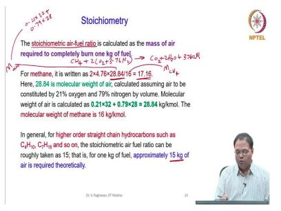
Now, another definition is stoichiometric air fuel ratio is nothing, but the mass of the air required to completely burn one kg of fuel. Now, we have found what? The number of moles required to burn 1 mole of fuel.
