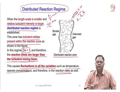
The third regime is called distributed reaction regime. Here, the length scale ratio is smaller and that relative turbulent intensity is large, that is this. Now, we get that distributed reaction zone which is established.
