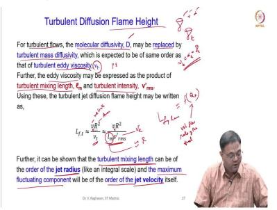
Now, turbulent jet flame height, we have seen it to be constant. Let us do the scaling analysis. We have done the scaling analysis for the laminar regime, where we have clearly seen that the flame height in the laminar regime is a function of  $Q_F$ ; this is the volumetric flow rate of the fuel.
