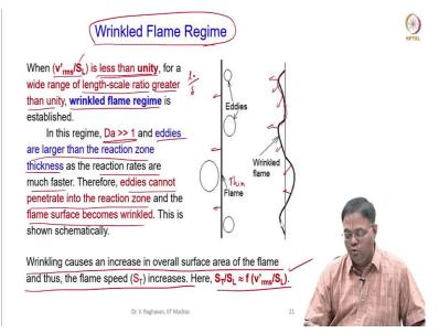
In the first case, what we have seen is less than unity; turbulent intensity is smaller, laminar flame speed is higher. Now, I increase the intensity, so that it becomes greater than unity. So, in that ratio for example, for the same range of the length scale ratio, what we saw in the wrinkled flame regime. The previous regime what will be the range of the length scale ratio. This is this same range what we saw in the wrinkled flame, the same range you get this.
