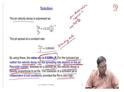
Whereas, in laminar jet the velocity decay is directly proportional to the Reynolds number; but for turbulent jet neither the velocity decay nor the spreading rate depends on the Reynolds number, it is not depending on the Reynolds number.
