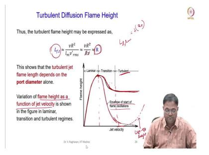
So, when I do that,  $v_e$  I substitute. So, this cancel and I get R. So that means, the turbulent flame height will depend only on the port radius that is what we have also seen there. So, in the turbulent case, analytical solution what we have seen here. You can see that the epsilon is function of  $v_e$  and R and here also you can see that there is no velocity decay or the spreading rate does not depend on the jet Reynolds number.
