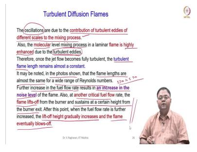
These oscillations are contributed by the turbulent eddies of different scale into a mixing process. So, at the non premix flame basically is set by a proper mixing of the fuel and the ambient air at stoichiometric proportions, where the flame zone is formed.
