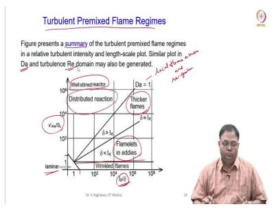
In summary, when we plot a map of the relative turbulent intensity and the length ratio  $l_0/\delta$ , I know that this is the log of scale, this is say 10. So, when both these quantities are less than 10, you get regime which is laminar, which are phenomenal laminar. Then, the wrinkled flame as I told you the turbulent intensity is very low and for a given range of length ratio, I get wrinkled flame; very low turbulent intensity.
