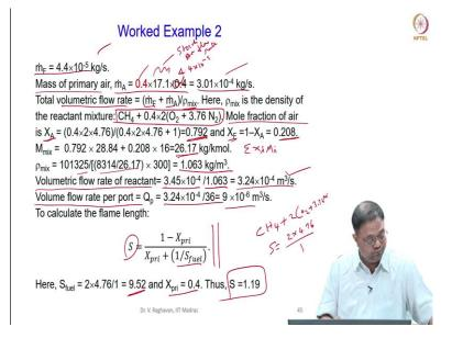
Then mass flow rate of oxidizer, I want 40% primary air. So, I know this 17.1 is the stoichiometric air flow rate. See for 1 kg of methane, I need 17.1 kg of air.
