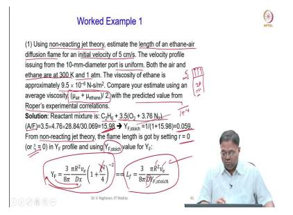
So, let us see couple of worked examples The first one is using non reacting jet theory; we have already seen the non reacting jet theory. Let us estimate the length of ethane air diffusion flame, initial velocity of 5 cm/s. Please understand that I do not need reactions at all for a diffusion flame, pure diffusion flame I do not need. Just by analyzing the non-reacting jet theory, I can find the flame length.
