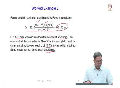
Now, substitute this in the correlation, Roper correlation; you know the  $Q_F$  for individual port that is  $9 \times 10^{-6}$  m<sup>3</sup>/s. T<sub>F</sub>, T<sub>∞</sub> are 300 K. Then 1n(1 + 1/S),  $1/S_{fuel}$ . So, 19.6 mm. You get flame length as 19.6 mm, which is less than the constraint given, 20 mm, that is fine.
