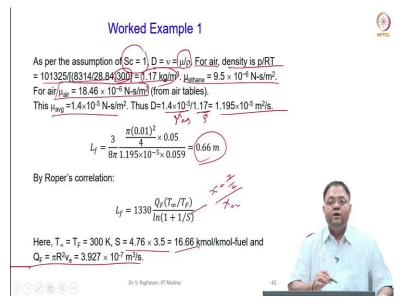
Now, again go for the assumption which we already made in the theory. So, v = D. So,  $\mu/\rho = v$ , so that we will do. So, nu, mu is nothing but the average which is given here. So, for air, first we will calculate the density by p/RT; p is atmospheric pressure, 1 atm. It is divided by molecular weight of the air is 28.84. So, the specific gas constant is 8314 by molecular weight into temperature, so the density is 1.17 kg/m<sup>3</sup>.
