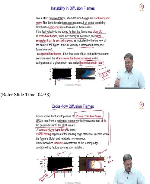
So, as I told you in this stable crossflow flame here, you can see a boundary layer formed, this is the leading edge of the fuel injector; a flame is formed very close to the leading edge of the fuel injector and it goes like this.
