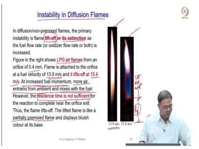
Now instability in diffusion flames. The possible instabilities we have in the diffusion flames is only one; that is liftoff and subsequent extinction. Again, I am given the example of the LPG jet flame. You can see that, this LPG jet flame is coming out from a very small orifice what we see in a Bunsen burner, it is about 0.4 mm orifice.
