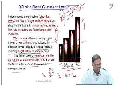
So, if you see all the flames what we have depicted in these figures, we can see that this is the radius so, the flame radius is almost of order of, it is not exactly equal to the radius, but of order of the radius of the port. If you have a bigger pipe, then the flame also will be bigger, the flame radius will be at least equal to the radius of the pipe.
