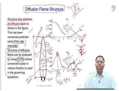
You can see that it is almost consumed. It is not like exact 0, this is fuel and oxidizer it is not exact 0 here, it will be like this small leak will be there due to some thickness. So, if it is exact 0 like this, then the flame will have 0 thickness here like this. But it is not exact 0 here, it goes to 0 slightly away from this.
