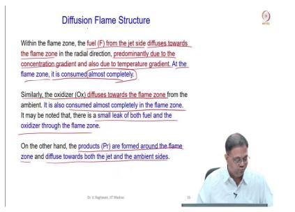
So, that is what we are trying to put up here. You can see that within the flame zone, fuel on the jet side diffuses towards the flame zone predominantly due to concentration gradient and temperature gradient. At the flame zone the fuel is consumed that means, at the flame zone where the maximum temperature occurs, the products are formed the fuel is consumed.
