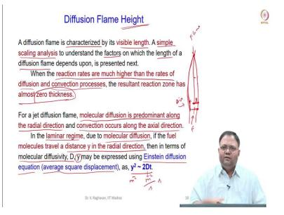
Now, as I told you very important characteristic of a diffusion flame is the visible length or the height of the diffusion flame. So, how to calculate that?
