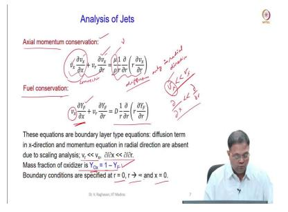
So, there is no time dependent terms involved in this. Similarly, axial momentum equation  $v_x \partial v_x / \partial x$  convective term plus  $v_r \partial (v_x) / \partial r$ . So, the axial momentum conservation so,  $v_x$  is the convective term here.
