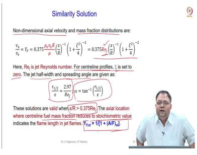
Now, if you want to plot here, so, non-dimensional axial velocity and mass fraction distributions are given here, basically this is the  $v_x/v_e$ , which is equal to  $Y_F$ , that is the profile here.
