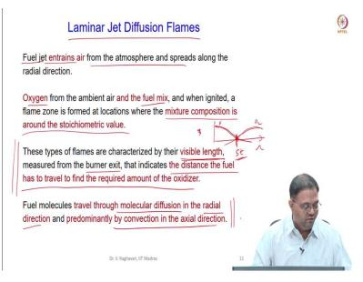
So, laminar jet diffusion flames. So, fuel jet which is coming out with some momentum which will entrain the air due to the viscous effects, what we have saw after the potential core region, you can see that the viscous effect will be more and the mixing takes place
