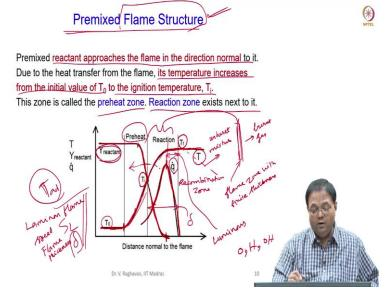
Now, we are interested in finding two things; the structure basically, also we are interested mainly to find this S<sub>L</sub> value, associated with this is the thickness of the reaction zone which is called  $\delta$ ; so, del. So, laminar flame speed and flame thickness and  $T_{ad}$ ;  $T_{ad}$  is thermodynamically you can find this. So, this is not a problem. Then the structure, basically we are interested in the structure. So, these are the important things.
