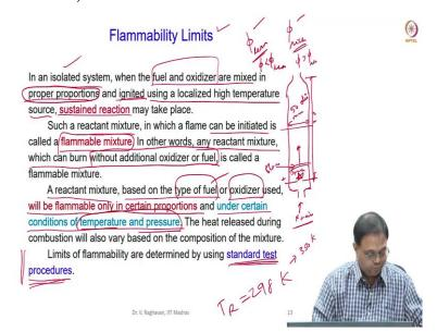
So, I say fuel plus air is supplied here, you can have any reactant. Please understand that fuel plus oxygen also you can supply; any reactant at any temperature, you can make and supply this and once this is filled up, then give a spark here and see whether a flame is formed. So, once you give a spark, a flame forms.
