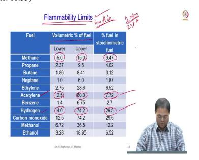
And this is the table of flammability limits of several fuels, important fuels are given here and please understand that here we have not presented it as a function of  $\Phi$ ; but I have given volumetric percentage of fuel, when I have a fuel air mixture and this is for the air, flammability limits in air. If it is in oxygen, it will be different. So, this is in air and one more thing is this is conducted at one atmospheric pressure and 298 K, that is the initial condition of the reactants.
